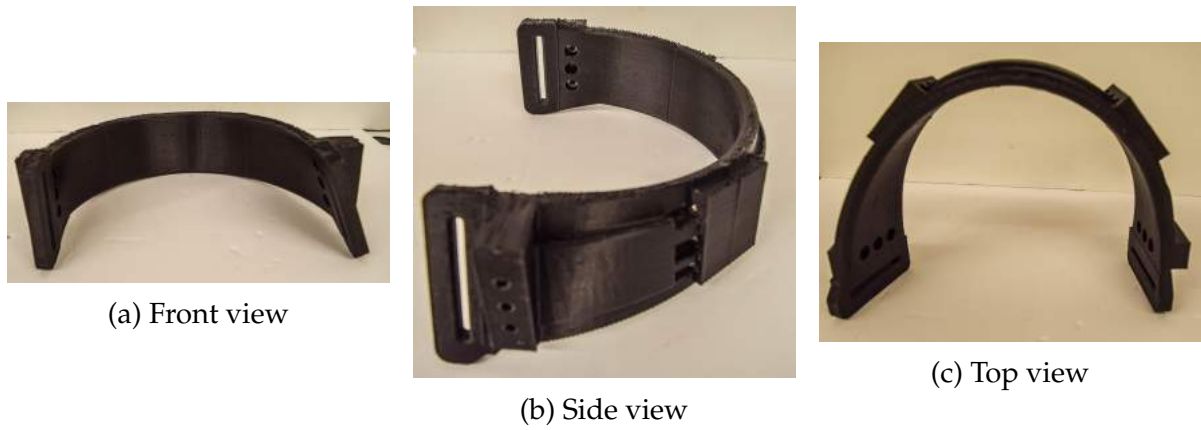
Figure 3.13: Different views of the posterior thigh interface
