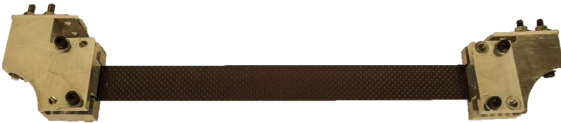
Figure 3.5: Elastic element composed of clamping brackets and the carbon fiber strip
