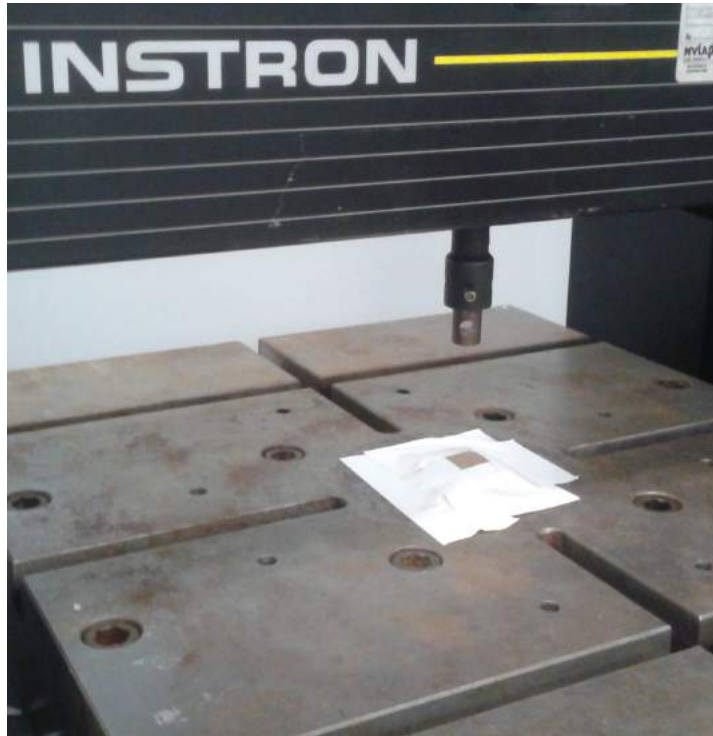
Figure 4.4: Calibration interface made of multiple layers of rubber sheets. These layers are held down on the platform with white tape.
