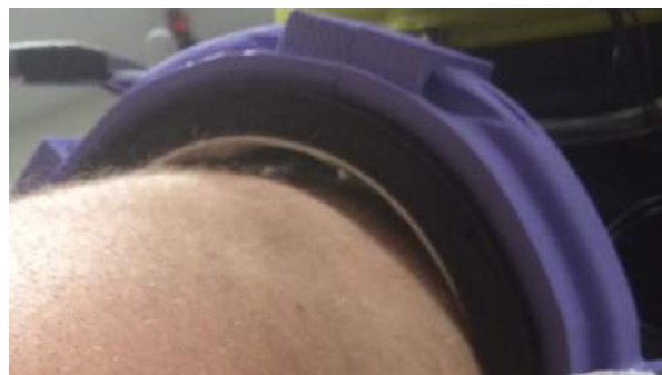
Figure 5.30: Loss of interface contact could visually be seen
