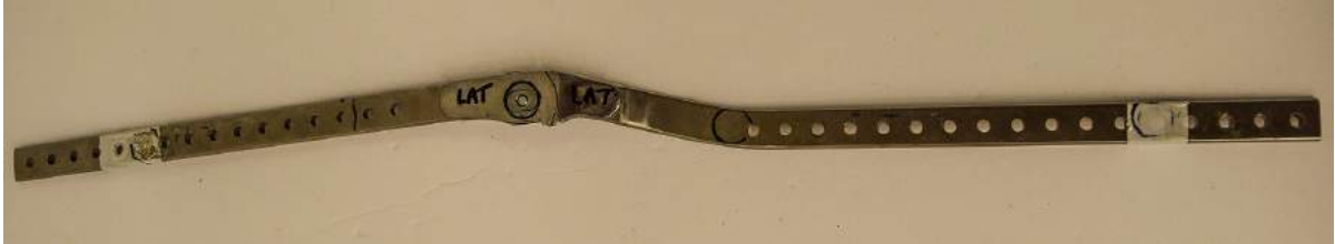
Figure 3.2: Stainless steel orthotic uprights
