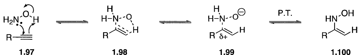
Figure 1.2. Cope-type Hydroamination: General reaction scheme and mechanism.
