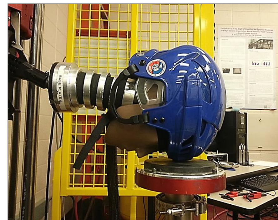
Figure 1. Youth headform, linear impactor Figure 2. Adult headform, monorail
