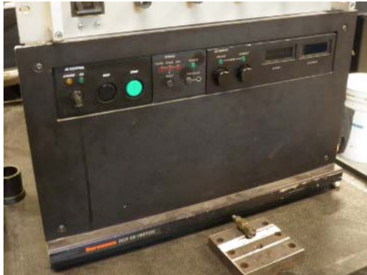
Figure 4.9 : 10kW Powder supply to heat the coil
