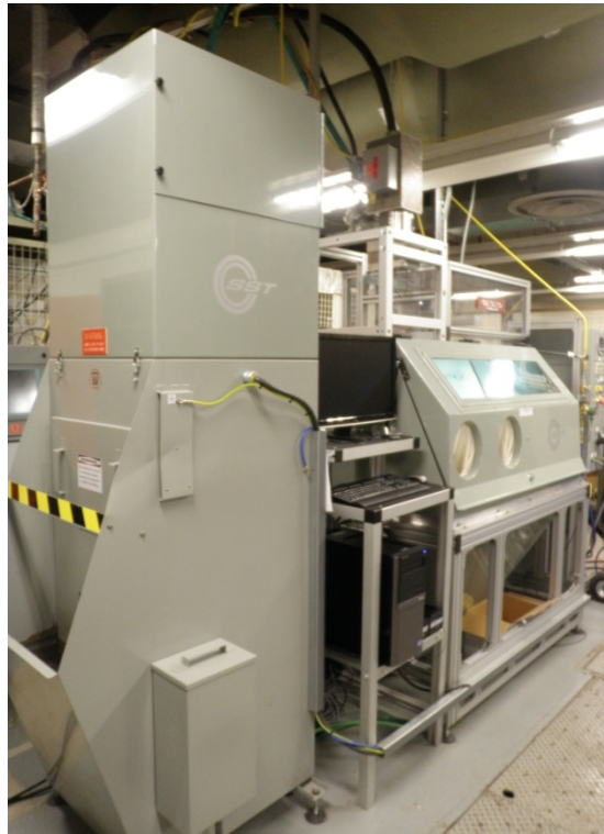
Figure 4.12 : Spraying chamber and water filtration unit
