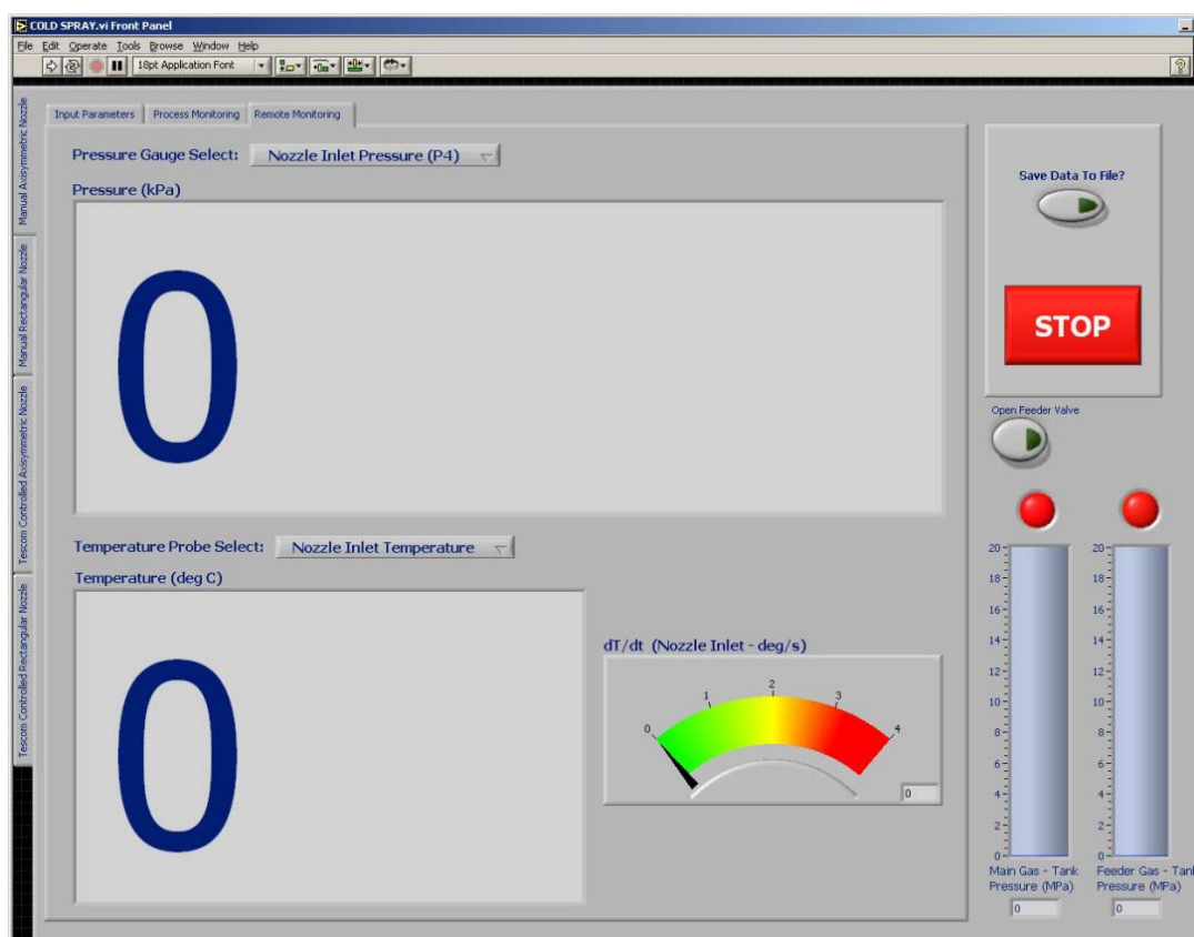
Figure 4.4 : Screenshot of Labview interface computing pressure and temperature parameters
