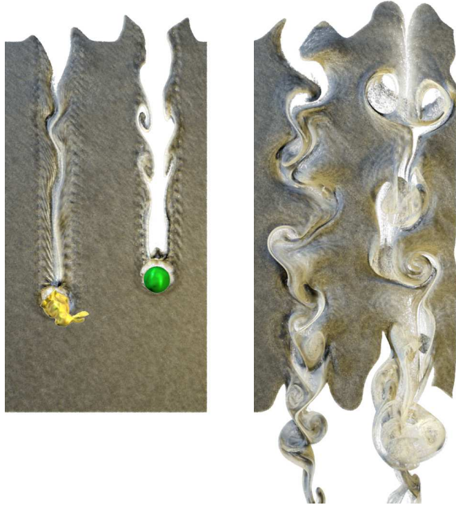
Figure 7.2: Simulation snapshots of different patterns of vortex shedding produced on a sheet of smoke by a bunny model and a sphere. An animation sequence for this figure is shown in the accompanying video at 0:05.
