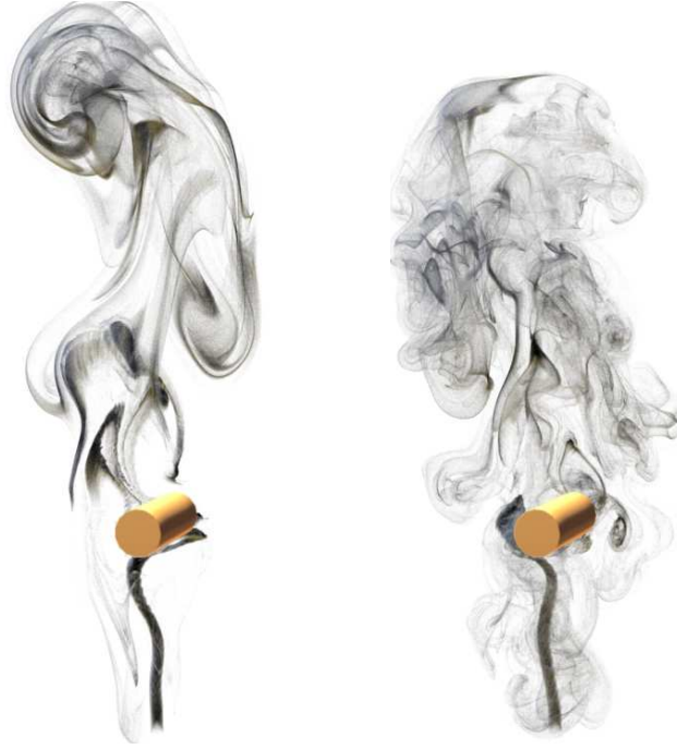
Figure 5.7: 3D flow pattern comparison with a vertical vortex jet around a static cylinder of unit radius with slip coefficients c = 0.0 (left) and c = 1.0 (right). An animation sequence for this figure is shown in the accompanying video at 1:28.
