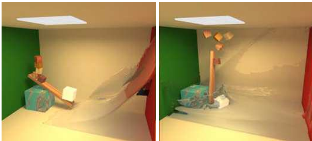
Figure 3.15: Animation frames of interaction of solids and fluids in Carlson et al. [19] a liquid is advanced from the right, collides with some solid objects which move due to the fluid motion and these in turn alter the motion which is noticeable in the lower part of the scene. Reprinted from Carlson, M., Mucha, P. and Turk, G. “Rigid fluid: animating the interplay between rigid bodies and fluid,” ACM Transactions on Graphics (TOG) - Proceedings of ACM SIGGRAPH Asia 2004, Vol. 23:3, © 2004 ACM, Inc. http://doi.acm.org/10.1145/1015706.1015733 .
