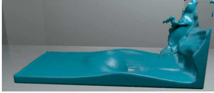
Figure 3.1: Results of liquid simulation using adaptive mesh refinement using a tetrahedron discretization from Batty et al. [11] where the mesh ranges from 400K to 1.1M tetrahedra. Reproduced with permission from Batty, C., Xenos, S., and Houston, B., 2010. “Tetrahedral Embedded Boundary Methods for Accurate and Flexible Adaptive Fluids,” Computer Graphics Forum , 29 (2), 695- 704. © 2010, Wiley and Sons. Reproduced by kind permission of the Eurographics Association.
