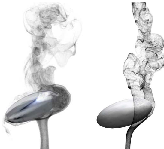
Figure 7.7: Left: Our results of smoke around an ellipsoid with vortex shedding. Right: Results for a similar scene from Weißmann, S. and Pinkall, U. “Filament-based smoke with vortex shedding and variational reconnection,” ACM Transactions on Graphics (TOG) - Proceedings of ACM SIGGRAPH 2010, Vol. 29:4. © 2010 ACM, Inc. http://doi.acm.org/10.1145/1778765.1778852 .
