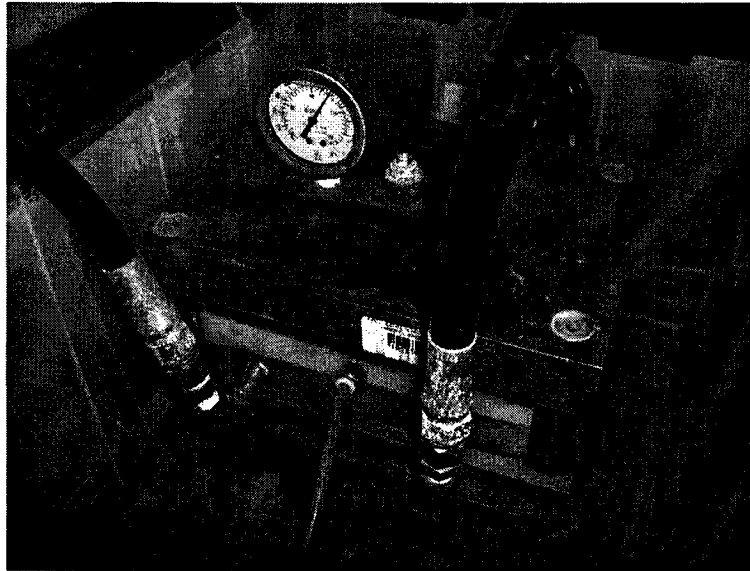
Figure 3 - 3 Osmonics Ltd. Sepa ® membrane cell with the inlet to the right, the outlet to the left and the permeate exiting the central hose.
