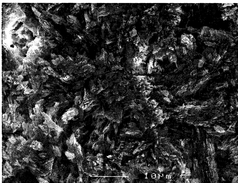
Figure 4-39 October 2, 2002 scale showing an overall flaky structure in SEM photo.
