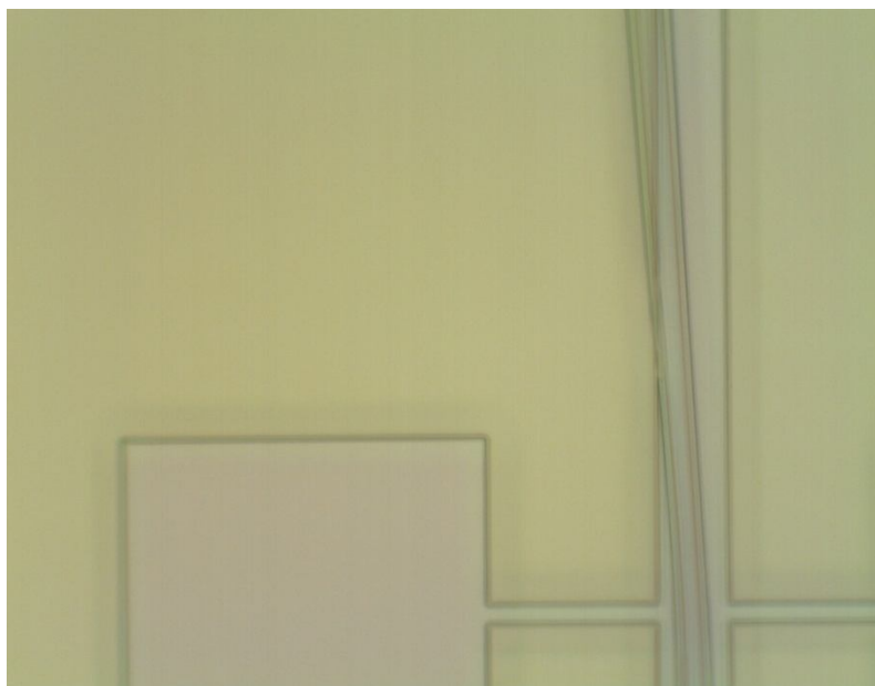
Figure 39 : Triple waveguides deformed due to overexposure to MF321. A) 10x magnification b) 100x magnification
