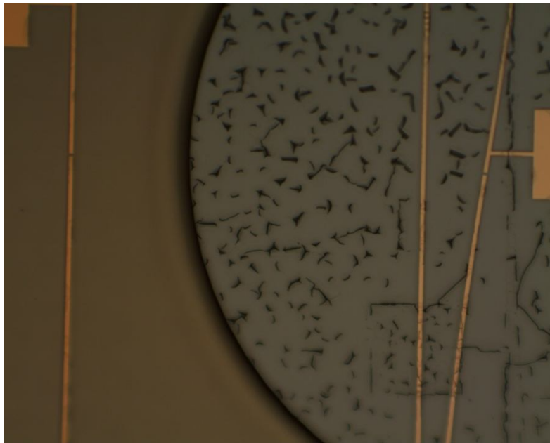
Figure 13 : Cracking of oxide layer due to aggressive O 2 plasma.
