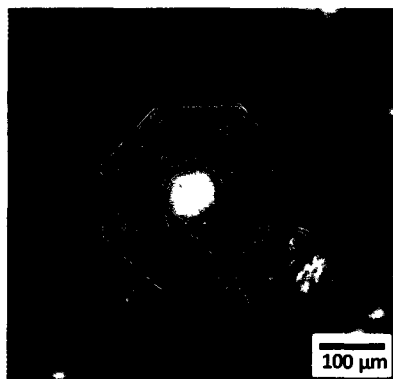
Figure 3.4: Rhenium gasket which has been preindented showing the shape of the diamond culet and drilled using electrospark erosion. The dark material surrounding the compression chamber is comprised of small molten globules of rhenium produced from the drilling process.
