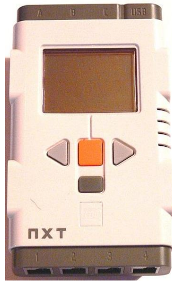
Figure 5.3 The NXT Intelligent Brick
