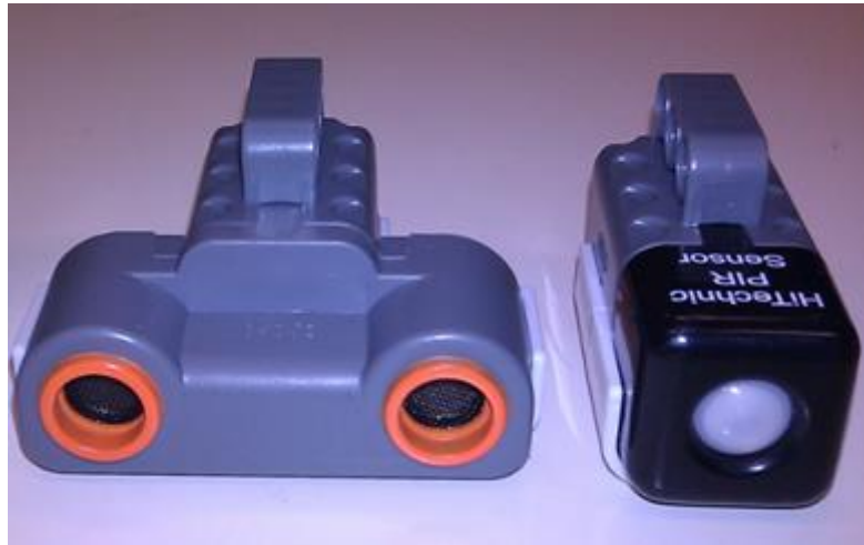
Figure 5.2 The ultrasonic sensor (left) and the human sensor (right)
