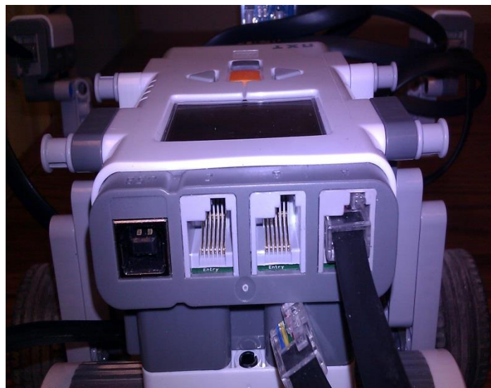
Figure 5.4 The interfaces of The NXT Intelligent Brick
