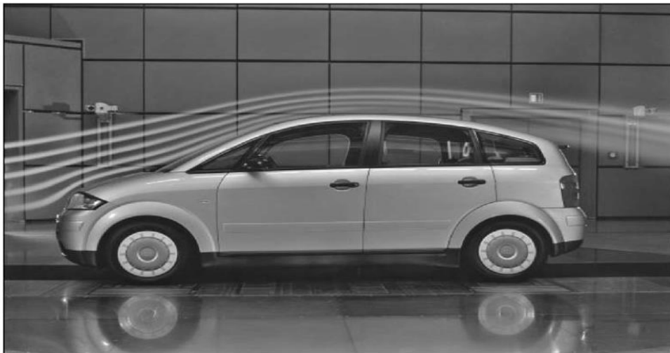
Figure 4.8 The streamlines of fluid flowing over an automobile in a wind tunnel [28]
