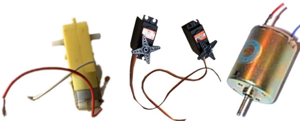
Figure 2.3: Examples of Actuators: DC and servo motor for use in applications to make a robot physically move or animate (Image created by Author).
