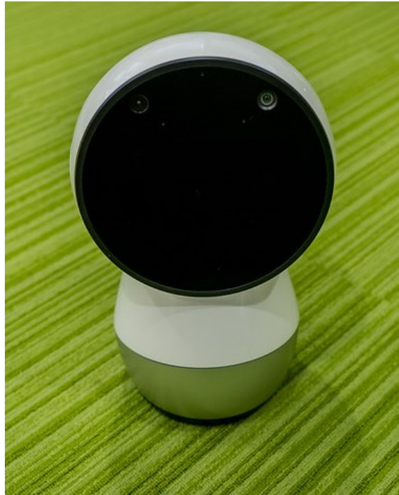
Figure 2.11: JIBO – A Social home robot with a 360 degree rotational body, intelligent voice commands and communication, and touch and facial recognition, which helps to create a genuine connection with its users. [21]. (Image CC under https://creativecommons.org/publicdomain/mark/1.0/ )
