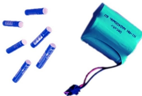
Figure 2.5: Examples of rechargeable battery power supply: Alkaline and Nickel Metal Hydride (NIMH) battery devices used for robotic design applications [93](Image created by Author).
