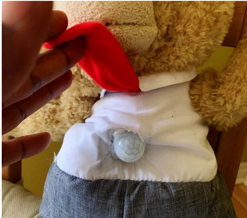
Figure 3.23: Representation and practical application of PIR motion sensor with the Teddy Bear robotic prototype (Image created by Author).
