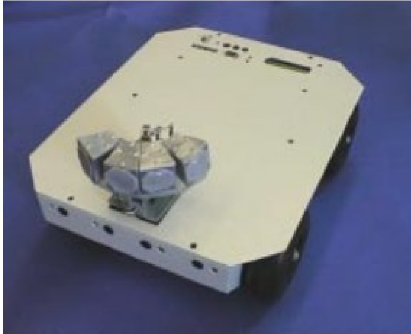
Figure 2.6: AURORA – The non-humanoid, truck-style robot platform used in the AURORA project, donated by Applied AI Systems, Inc in 1998 [114].
