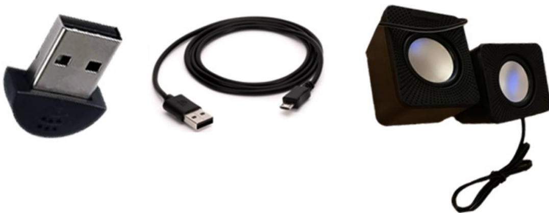
Figure 3.8: Peripheral devices: USB power cable, microphone and speaker used for power supply connection and voice communication with the prototype (Image created by Author).
