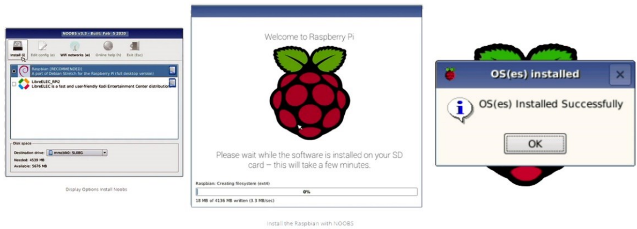
Figure E.1: Installation of Raspbian NOOBS OS on the RaspberryPi.
