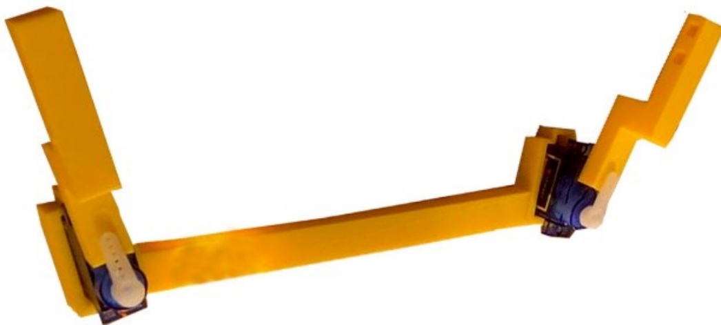
Figure 3.12: A 3D-printed robotic animatronics lever arm and with servo motors attached to cause robot arm to physically animate (Image created by Author).
