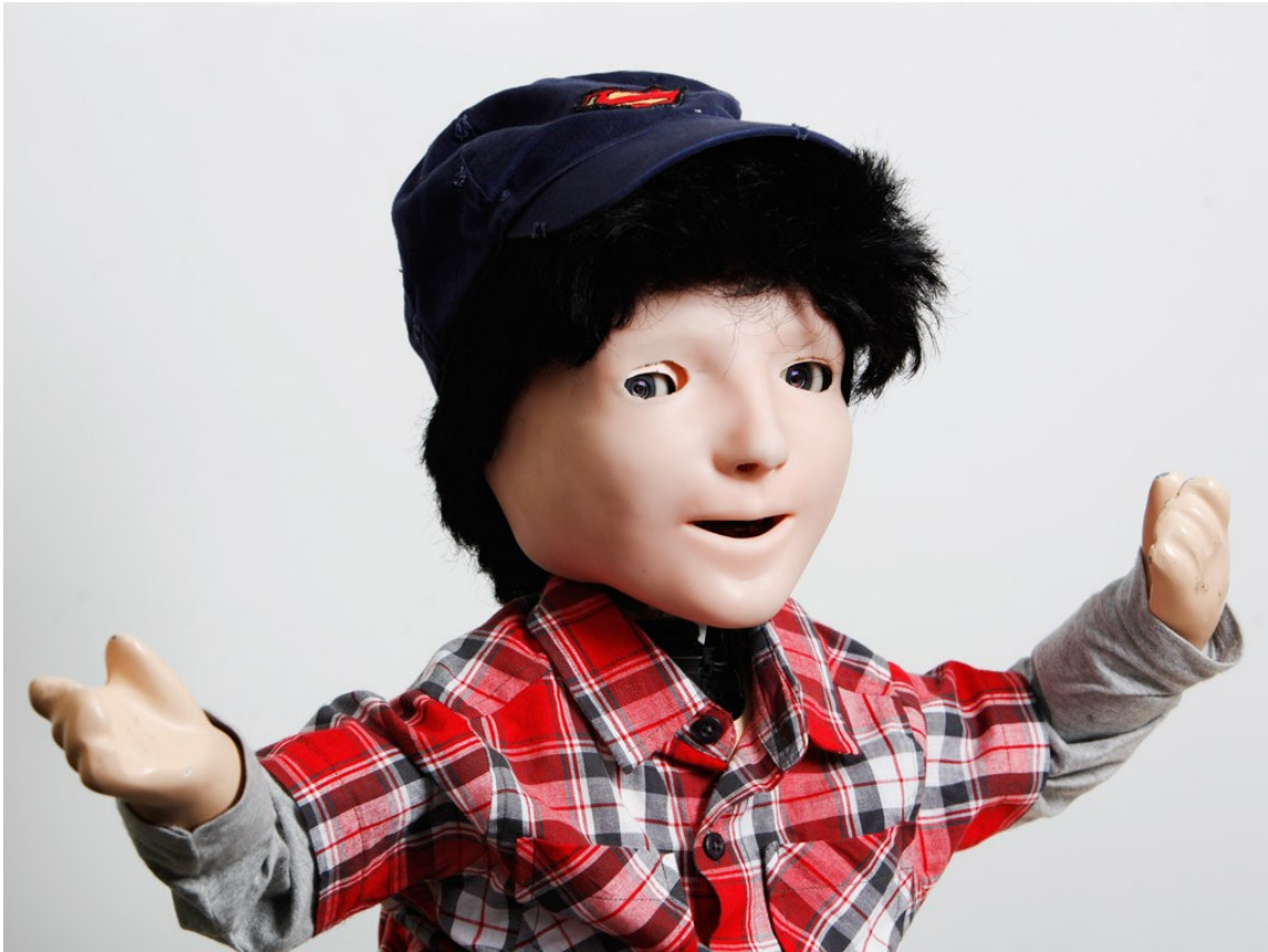
Figure 2.7: The humanoid robot KASPAR was designed with head and hands and includes touch sensors to detect objects around it; it also has microphone and speaker for communication [116] (Image under © Copyright 2020 IEEE - https://robots.ieee.org/robots/kaspar/ ).
