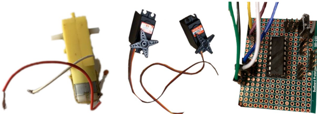
Figure 3.6: Robotic Actuators: DC and servo motors with L239D motor driver used in the robot's design to make it physically animate (Image created by Author).
