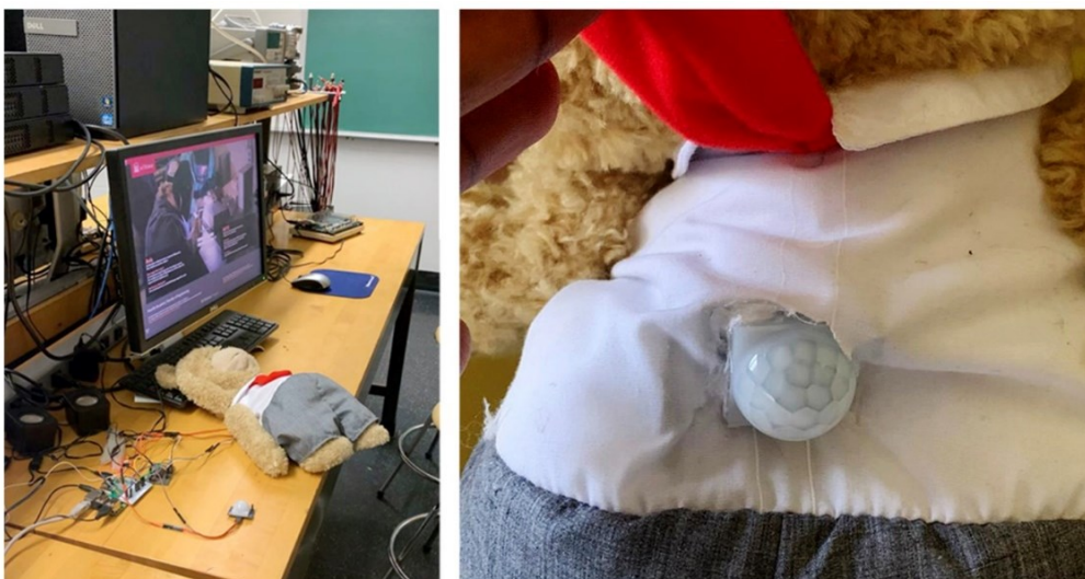
Figure 4.4: Laboratory testing and practical application of PIR sensor device state and attention model of the robot's prototype framework (Image created by Author).
