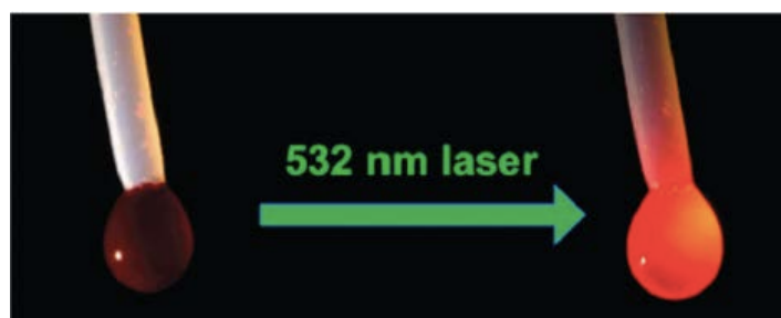
Figure 5.4 Pictures of the drop before (resazurin) and during laser excitation (resorufin); the bright point on the left of the drops is due to a reflection of the light source illuminating the drop, and the bright orange color of the right drop incorporates extensive product fluorescence.
