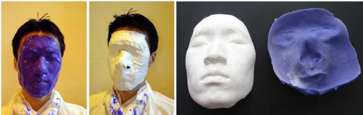
Figure 2.7: The process of constructing the negative and positive moulds of a human face (the results are in the right pane).
