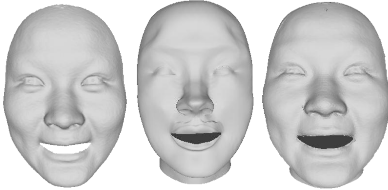
Figure 3.11: the left is input registered face with the deformed subdivided generic model in the middle, and the right face is the one after dense surface adaptation
