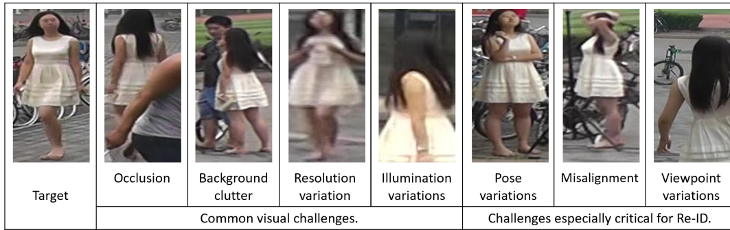
FIGURE 2.8: Examples of common visual challenges and challenges especially critical for person Re-ID, including occlusion, background clutter, resolution variation, illumination variations, pose variations, body-part misalignment, and viewpoint variations.
