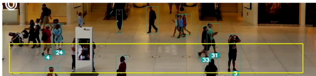
(E) Re-identification stage, where the pedestrians #42 and #44 are matched back to #31 and #33 respectively.
