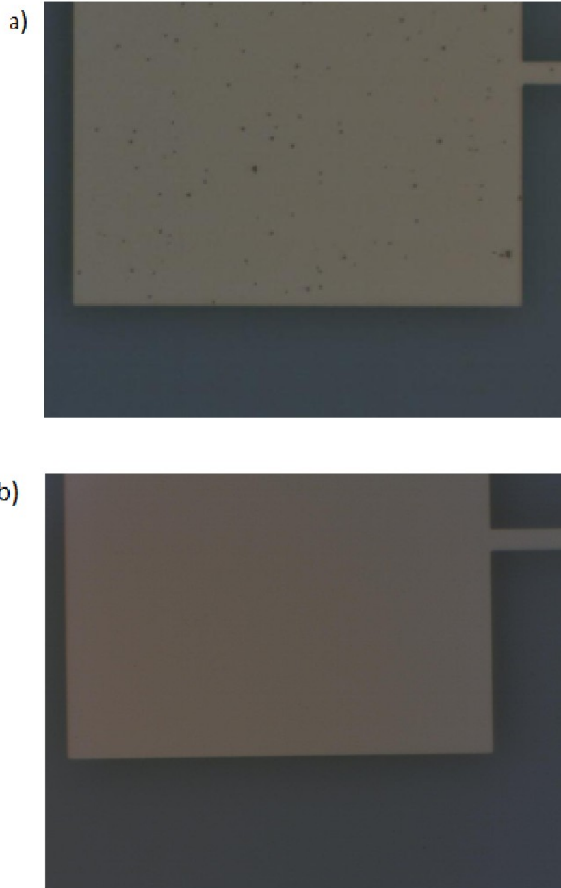
Figure 25: Gold contact pads after lift-off a) showing spits on surface using old deposition procedure [6], b) showing no spits on surface using modified deposition procedure.
