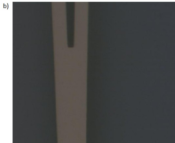
Figure 27: 2 micron Y-Junction of MZI, a) fabricated using LOR-1A lift-off resist, b) fabricated using PMGI SF 2G lift-off resist.
