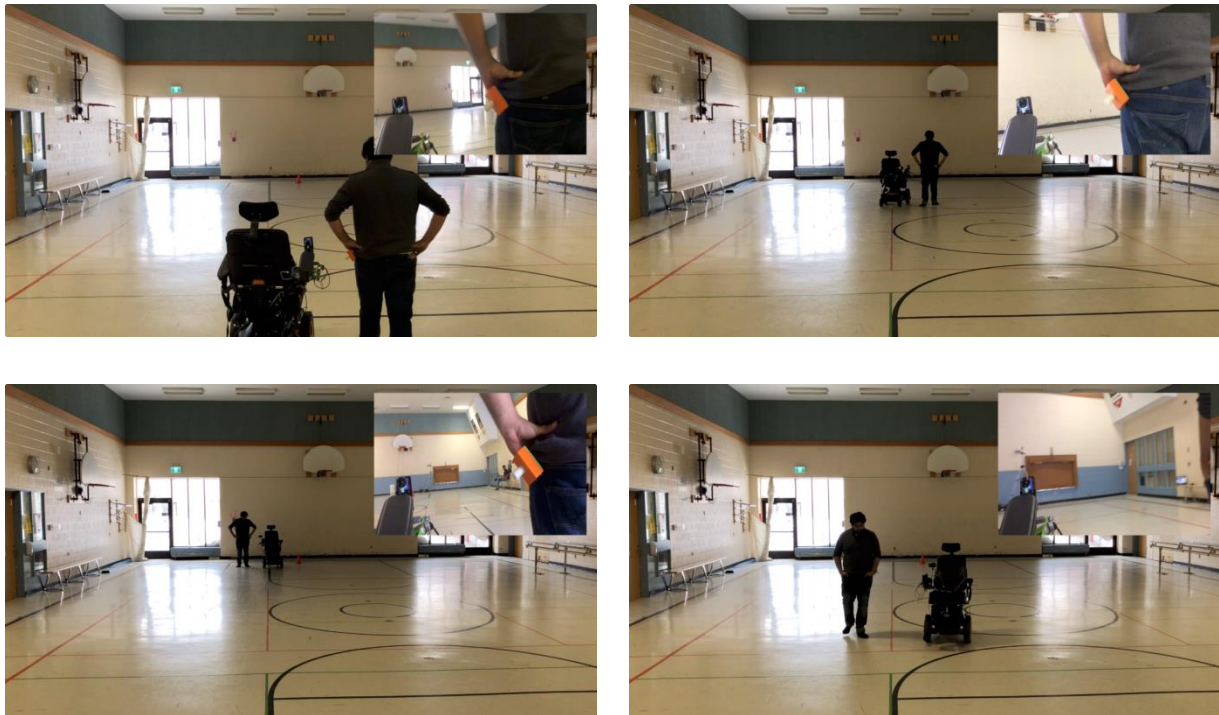
Figure 5.11 Processed video screenshots from the straight path test collected from a fixed camera (main video) and the smartphone camera mounted to the wheelchair (top right video overlay).
