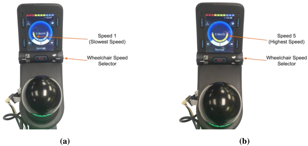
Figure 5.6 (a) Speed 1 (low speed) setting and, (b) Speed 5 (high speed) setting and the wheelchair speed selector interface on the manual joystick controller.
