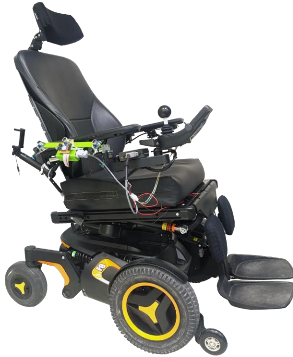
Figure 5.1 The ultrasonic tethering receiver mounted on a Permobil F3 Corpus wheelchair.
