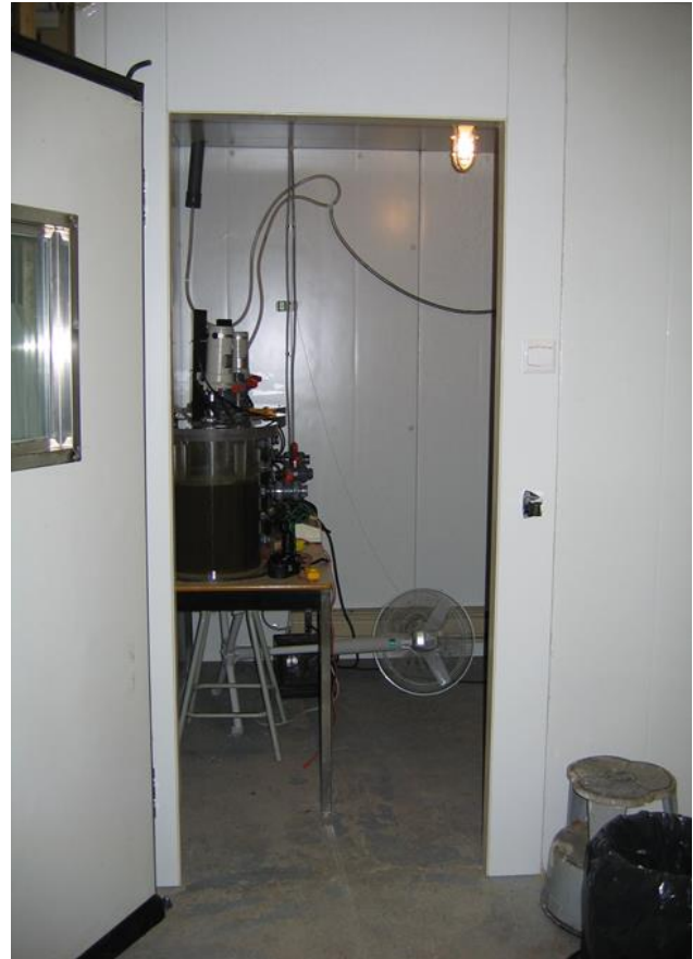
c) Heat Room for Mesophilic Incubation ( 36\pm 2^{\circ}\text{C} )
