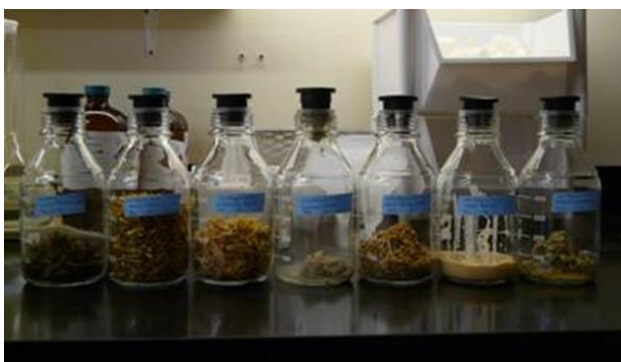
a) Prepared substrates for BMP assays in Wheaton Bottles
