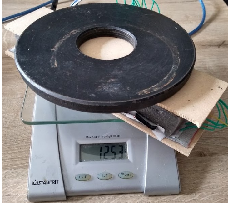
Figure 3.16: Calibration setup for pressure sensor matrices.
