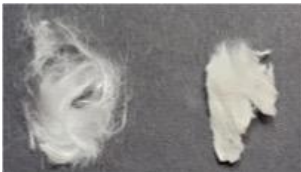
Figure 3.3.2. Close-up photographs of Glass wool alone, before the deposition of \text{TiO}_2 (left) and Glass wool after the deposition of \text{TiO}_2 (right).
