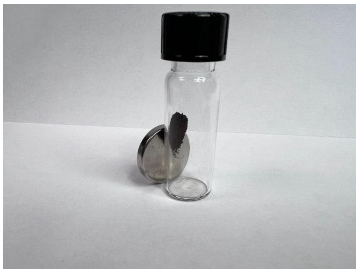
Figure 5.3.2. Fe 3 O 4 @TiO 2 after its synthesis next to a magnet to demonstrate its response to an external magnetic field.
