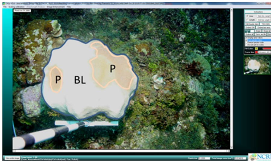
Figure 2.2.2. CPCe (Coral Point Count with Excel extensions) program provides a tool for image calibration and area analysis of benthic features. The traced circumference of a colony was used to calculate the planar colony surface area. Subareas within a colony area were used to estimate proportion of colony surface area that was fully bleached (BL), partially bleached or pale (PB/P), or recently dead (RM).
