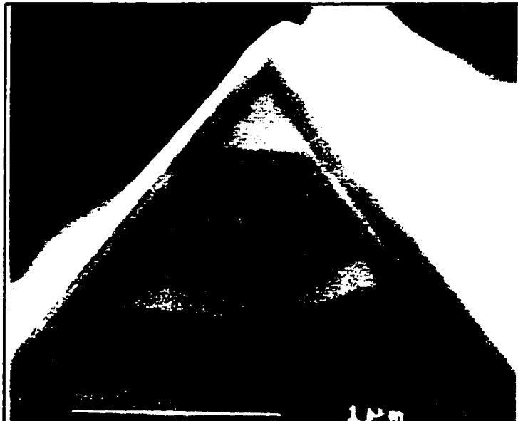
Figure 36. A completed V-shaped mesa InGaAs is light and InP is dark. The triangular light region is perhaps most striking. Note also the appearance of InGaAs on the (111)B sidewalls once the V is complete. The marker represents one micron.
