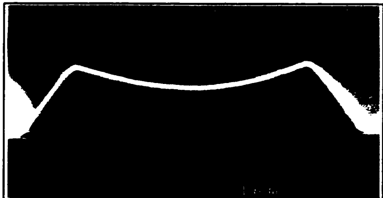
Figure 28. An [011] oriented InP mesa in cross-section.
