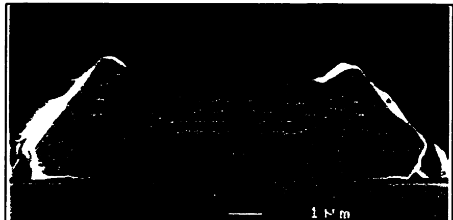
Figure 29. An [01\bar{1}] oriented InP mesa in cross-section.
