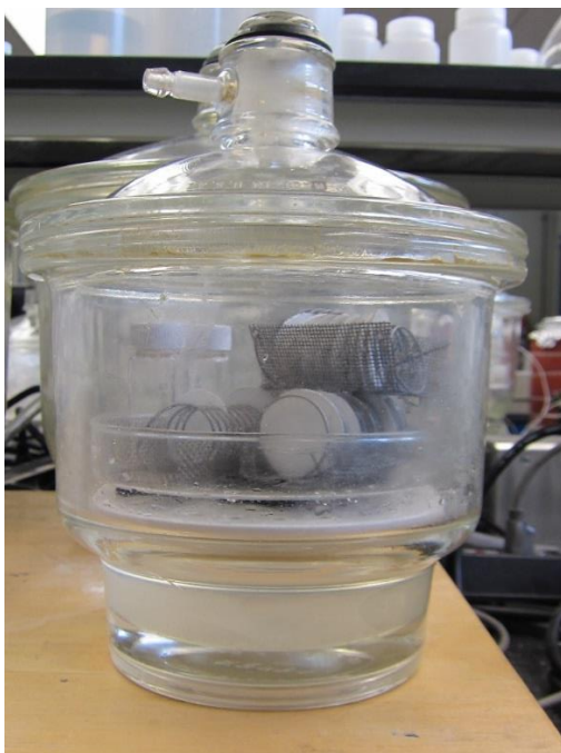
Figure 3.5: Vacuum-sealed desiccator conditioning samples at 11% RH.
