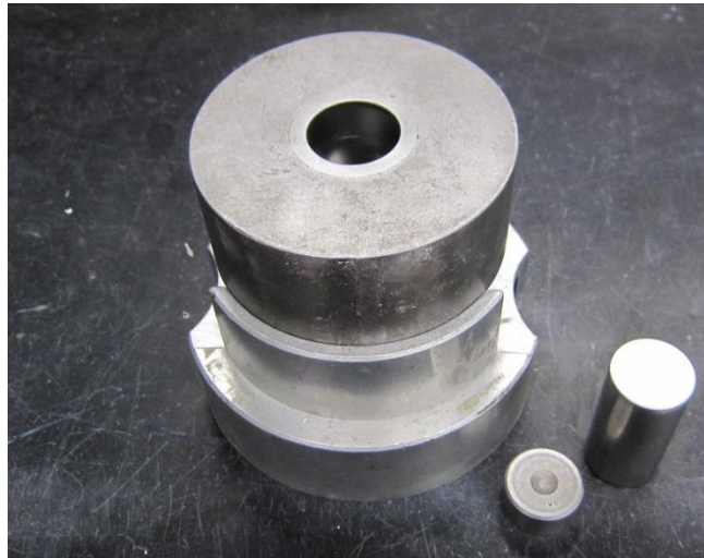
Figure 3.7: Steel mould used for pressure compaction
