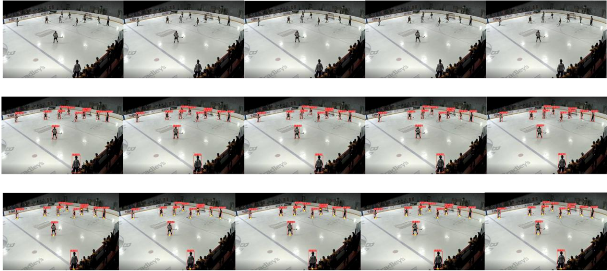
Figure 4-2. The first row displays five consecutive frames from a youth ice hockey game. The second row shows the corresponding frames with players detected using the fine-tuned YOLOv8 model, where bounding boxes are drawn around each player. The third row illustrates the midpoint of each bounding box, representing the player's estimated point of contact with the ice.
