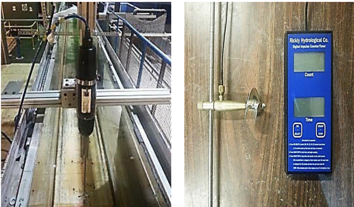
Figure 3-7: Instrumentation. a) Down looker Acoustic Doppler Velocimeter (ADV) installed over a metallic frame on the flume. b) Propeller meter.
