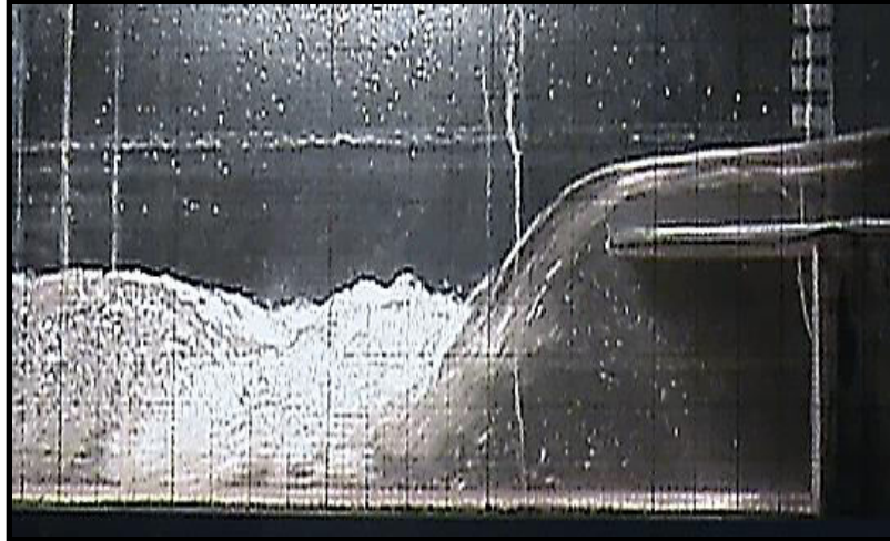
Figure 1-3: Submerged hydraulic jump experimentally simulated at the Hydraulics Laboratory at University of Ottawa.
