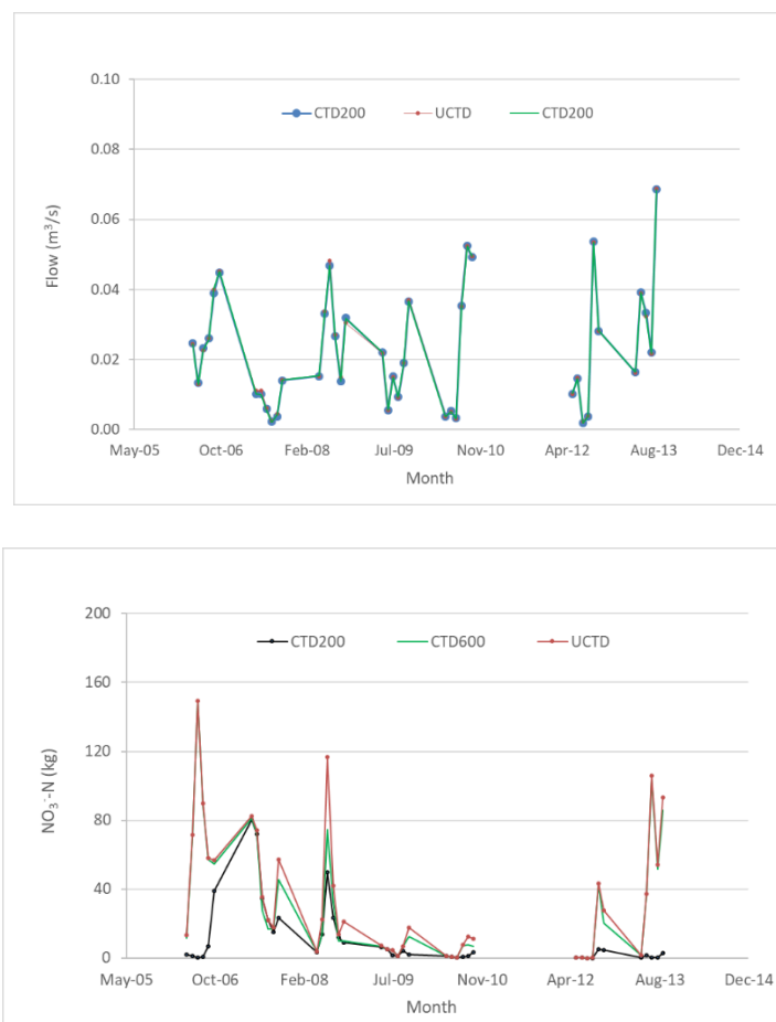
Figure 3.13 Simulated flow and \text{NO}_3^- -N for the CTD and UCTD scenarios using the CTD model
