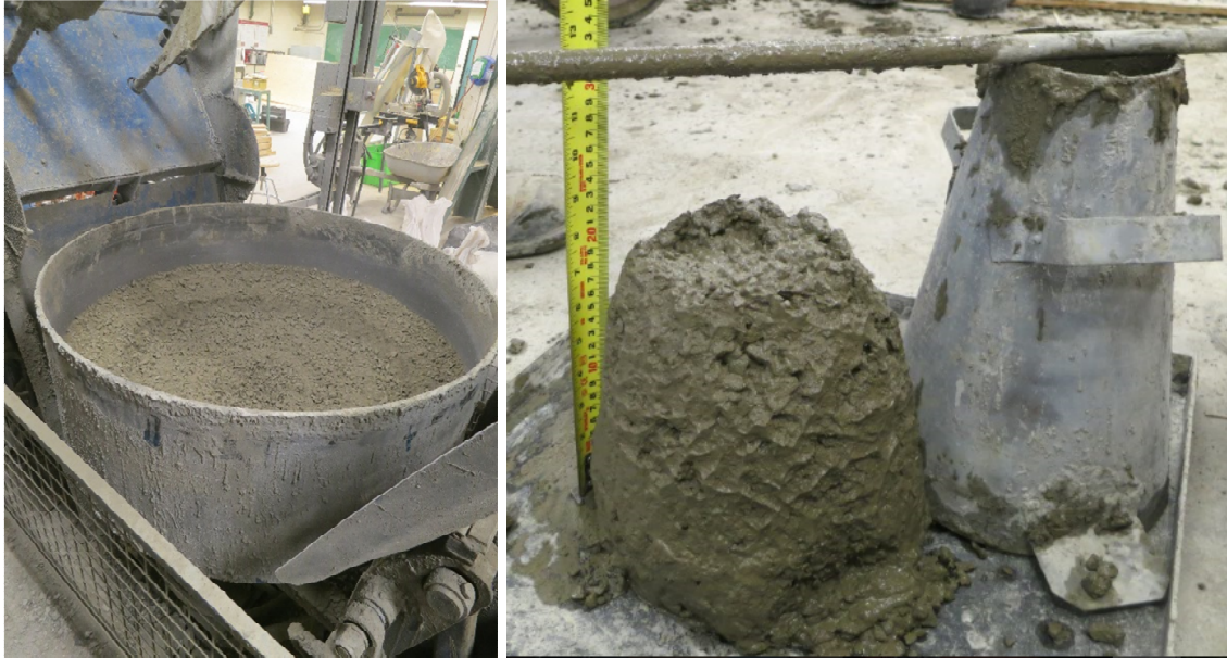
Figure 3-2 Normal Strength Concrete Mix
