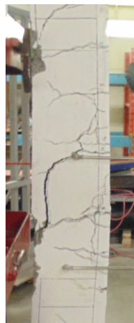
e) Mid-span cracking (south face) (Blast 3)
