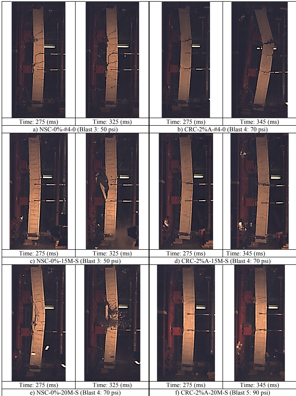
Figure 7-13 Debris and Fragmentation Control: Effect of Concrete Type
