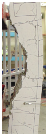
f) Mid-span concrete Crushing (South face) (Blast 4)
