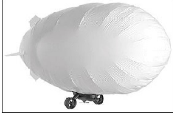
Figure 2.5: Tri-Turbofan has two thrusters oriented along the longitudinal axis for forwarding motion and a single thruster oriented along the vertical axis of the airship for altitude control [4].
