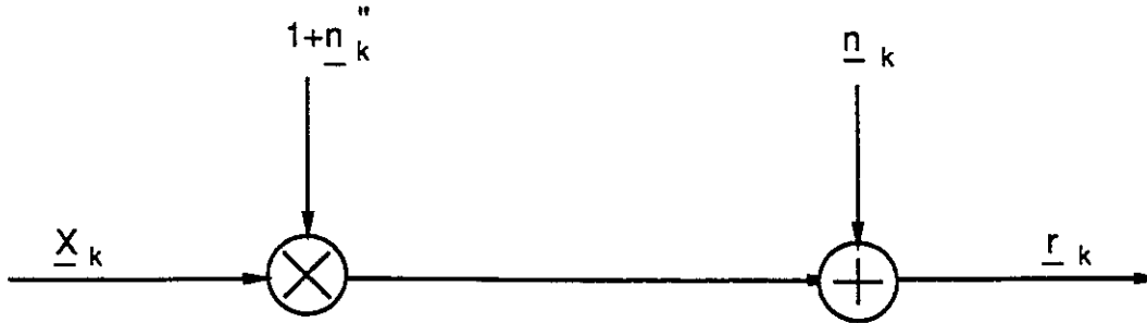
Figure 2.7: Complex baseband equivalent model of Rician Channels.
