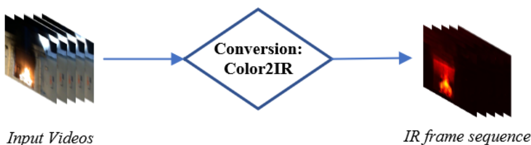
Figure 3-2: An illustration of the process of Color2IR Conversion. This module takes RGB videos as input and produces IR frames sequences.
