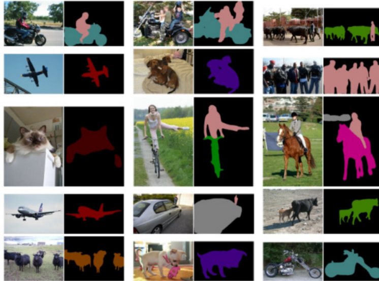
Figure 2-12: Semantic segmentation results. For each image pair, the left one is the original image and the right one is the segmentation results.
