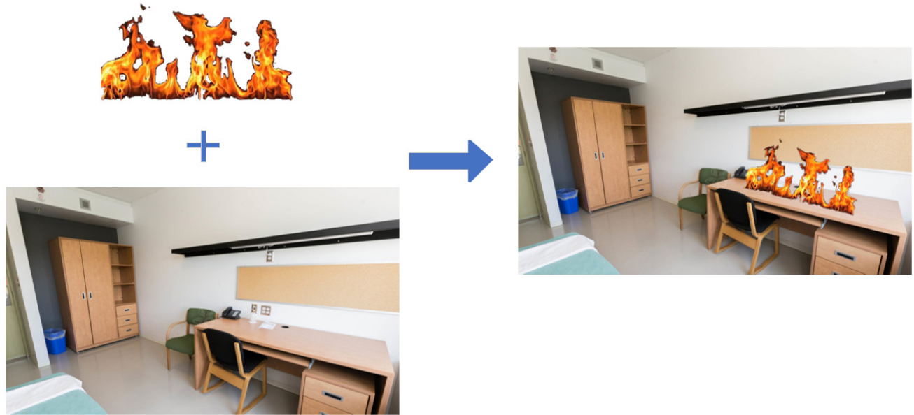
Figure 3-5: The generation of a synthetic image for data augmentation. The 2 images at the left are the source of the scene without fire and flame patterns. The flame pattern is superimposed to the scene for synthetic image generation.
