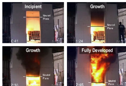
Figure 1-1: Examples of different stages of fire, from [4]. At 2:18, the size of the fire was not big yet, but at 2:45, the fire suddenly expanded.
