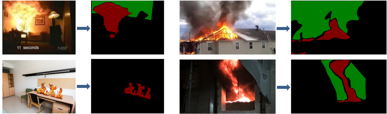
Figure 4-2: Samples and their annotations (red: flame, green: smoke) from the FS Segmentation dataset. The blue arrow indicates the direction of segmentation.
