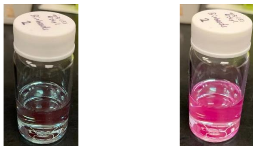
Figure 2.7 Solution of SiPz(Et 3 OSi) 2 in DCM under visible light (left) and irradiation with 254 nm UV light (right).
