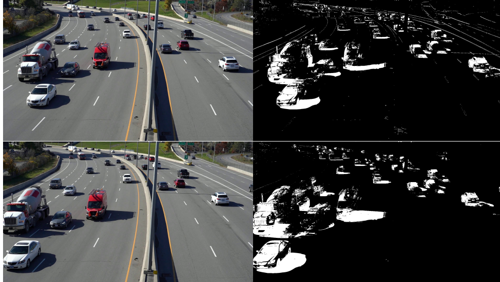
Figure 3.8: An example of a motion map generated using low-quality and high quality raw video. The resolution of the upper sub-figure is only 1280 \times 720 , recorded in a 5Mbps rate, while the resolution of the lower sub-figure is 1920 \times 1080 with 30Mbps bit rate
