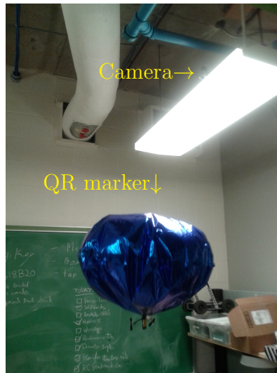
Figure 3.3: Airship during a minimum time linear displacement test.
