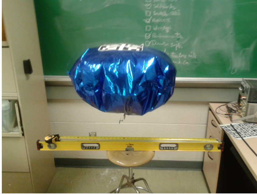
Figure 2.2: Airship during a minimum time linear displacement test.
