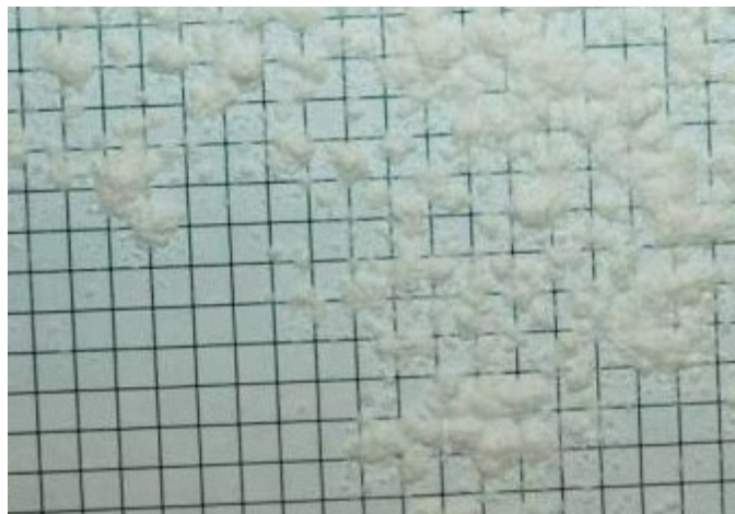
Figure 14: Solka-Floc Powdered Cellulose Sample (5x5 mm Grid)
