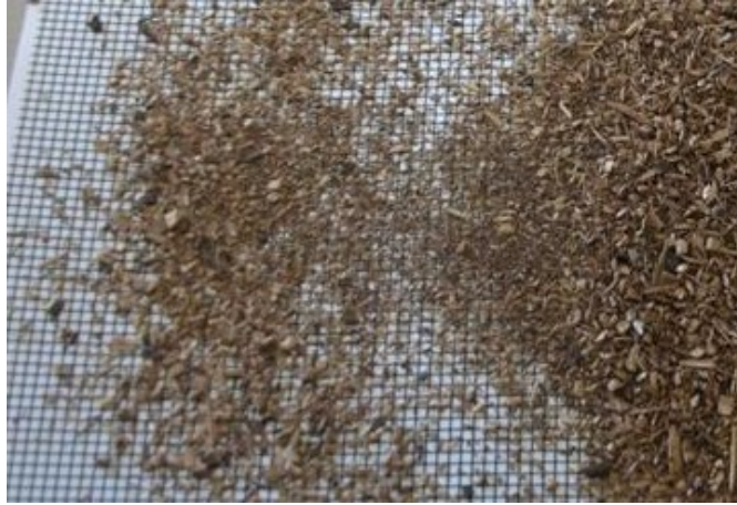
Figure 16: Interior Hog Fines Sample (2x2mm Grid)
