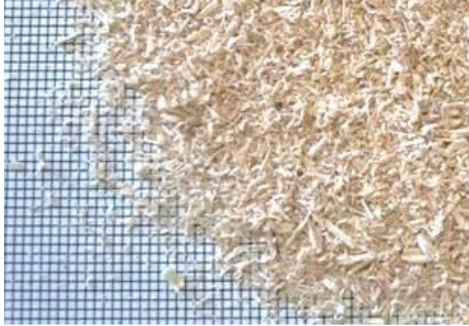
Figure 12: Hardwood Sawdust Sample (2x2mm Grid)
