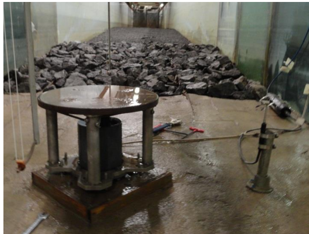
Figure 3.17: Model structure installed on top of force dynamometer in concrete pad
