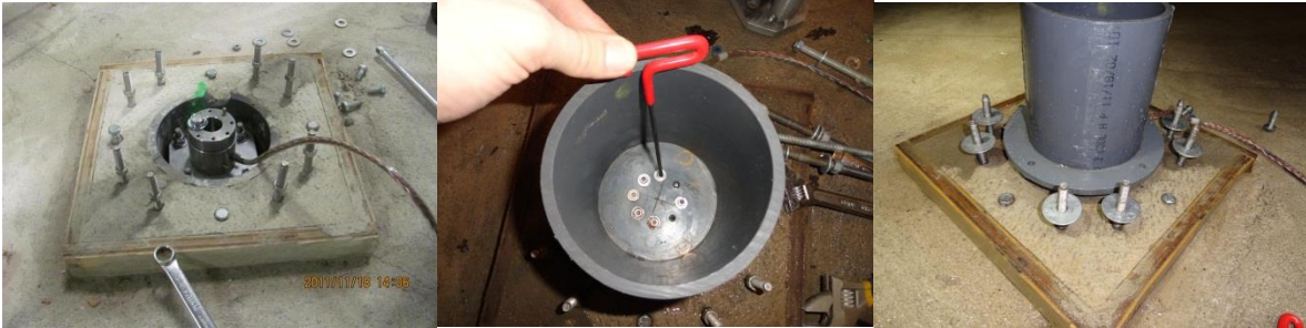
Figure 3.6: Images illustrating how the central pipe and ultimately the entire structure are supported by dynamometer
