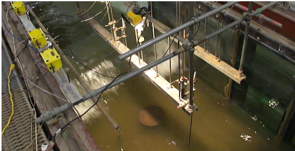
Figure 3.24: Freeze frame from filming of an irregular wave test (top view)
