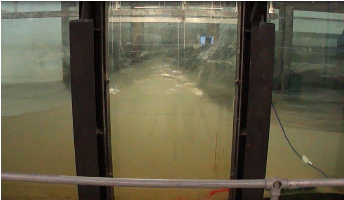
Figure 5.3: Side view of wave test 17 (+0 MWL, H_{m0} = 4.5\text{m} , T_p = 8\text{s} ) on full structure configuration
