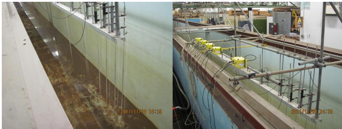
Figure 3.18: Array of 5 wave gauges in the deep water zone
