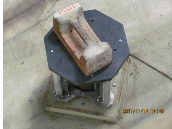
Figure 4.1: Calibrating the force dynamometer in the Z direction
