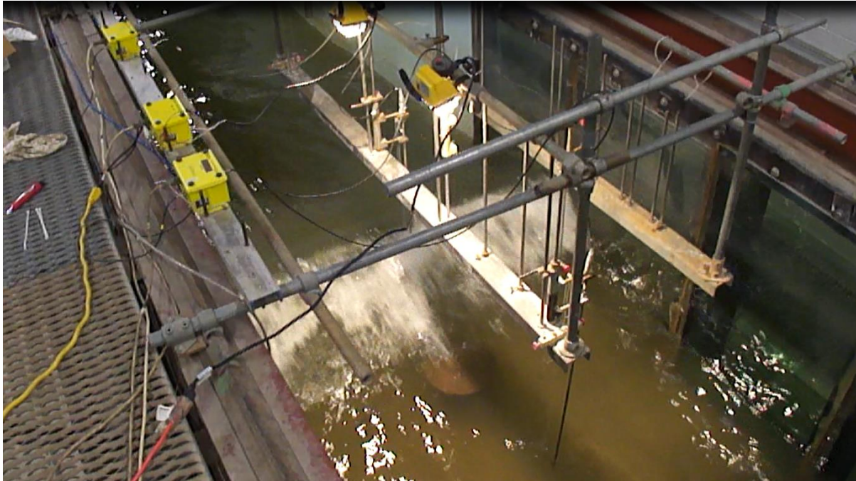
Figure 5.4: Top view of wave test 6 (-2 MWL, H_{m0} = 4.5\text{m} , T_p = 11\text{s} ) on full structure configuration
