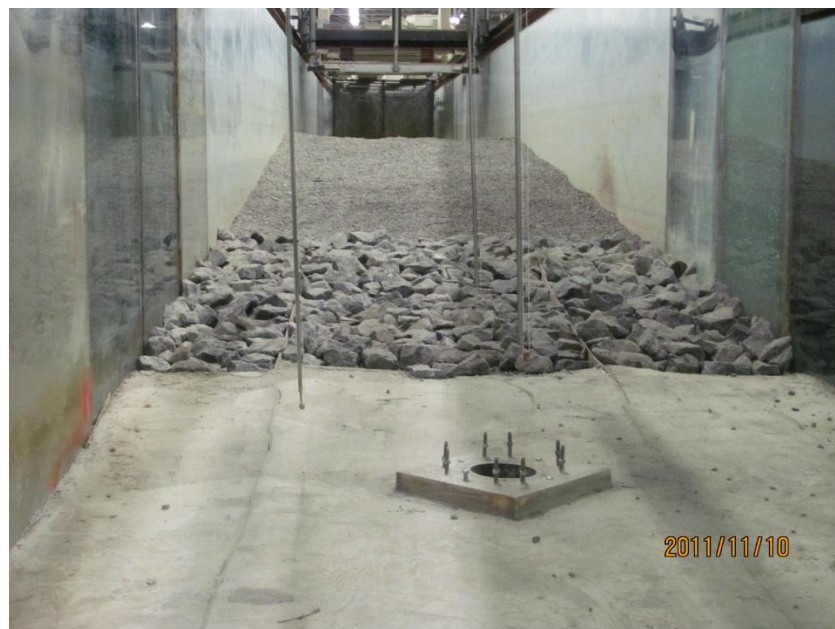
Figure 3.15: Finished bathymetry: concrete pad where structure will be fixed, large stone sea floor and pea stone beach
