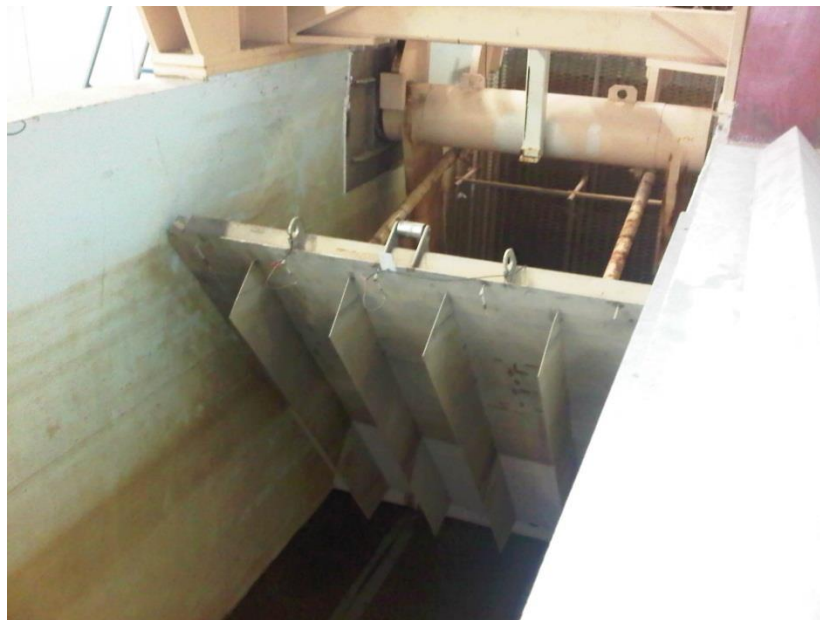
Figure 3.3: Wave maker at end of Large Wave Flume
