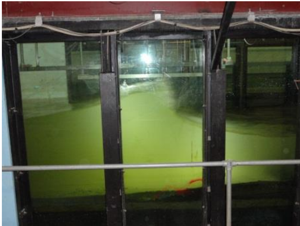
Figure 3.2: Observing a breaking wave through viewing windows
