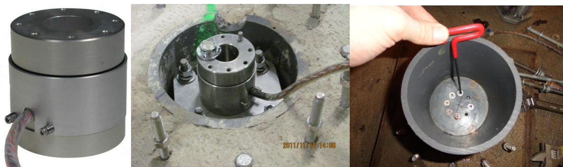
Figure 3.21: 6-axis force sensor used during testing on the model structure
