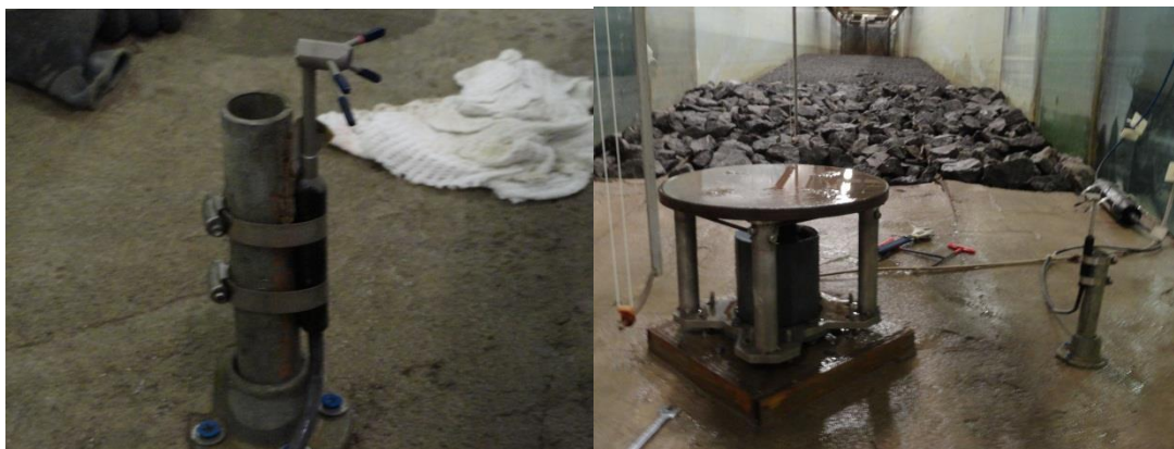
Figure 3.22: The Vectrino acoustic velocimeter mounted to face the model intake structure
