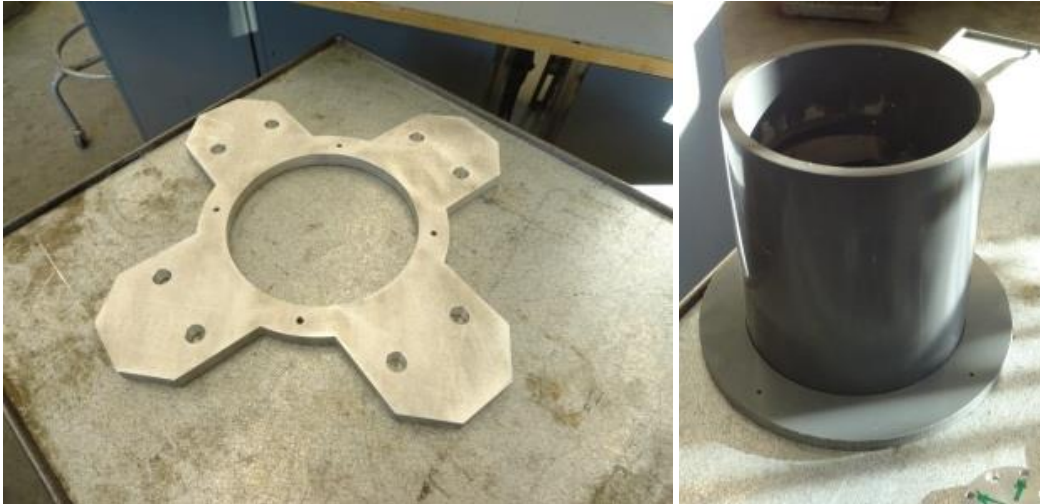
Figure 3.5: Pipe and posts aluminum base plate (left); Central pipe with PVS base plate (right)
