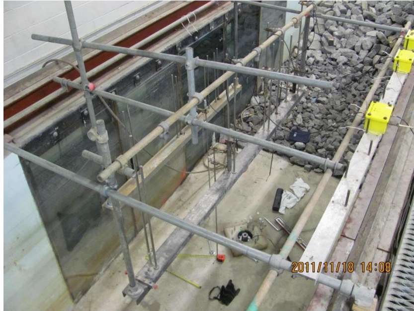
Figure 3.19: Set of 3 wave gauges in the shallow water zone at the structure location
