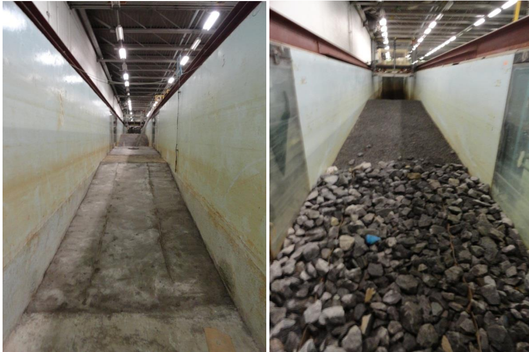
Figure 3.14: Left: finished concrete bathymetry viewed from deep water zone; Right: large stone sea floor and pea stone beach
