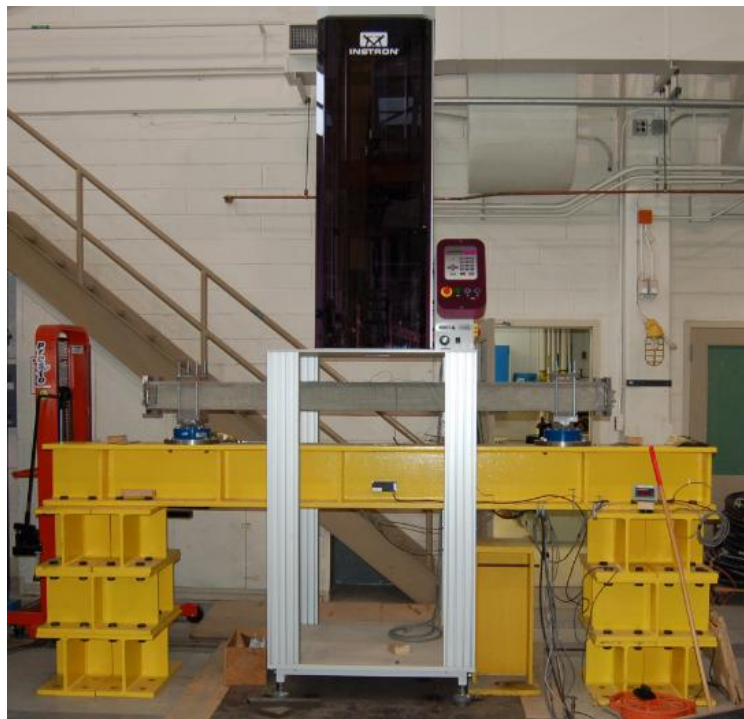
Figure 3-15: Ceast 9350 drop-weight impact tower with test specimen supported by custom supports installed on built-up frame
