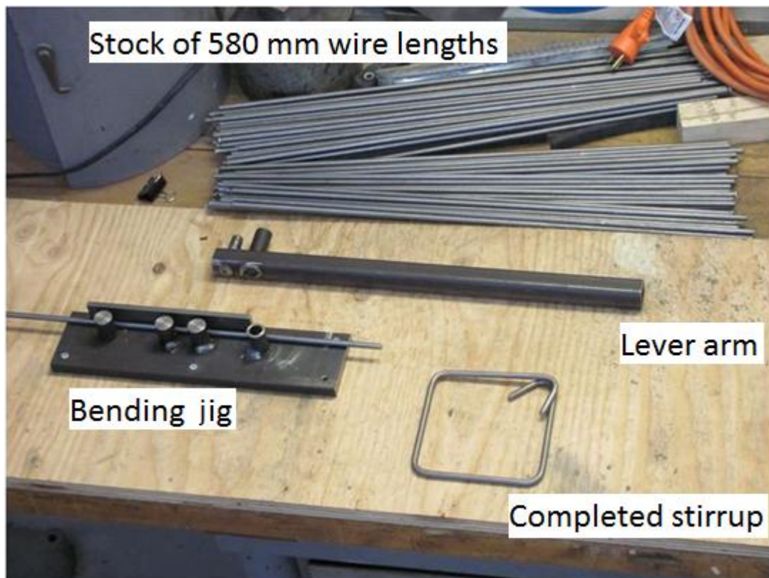
Figure 3-3: Stirrup bending jig, lever arm and completed stirrup
