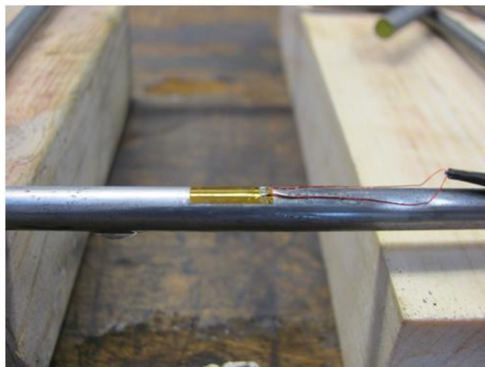
Figure 3-4: Strain gauge bonded to stirrup leg
