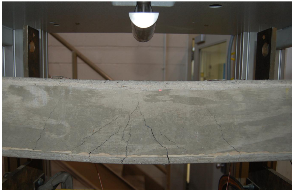
Figure 4-15: Impact zone damage for Imp-4
