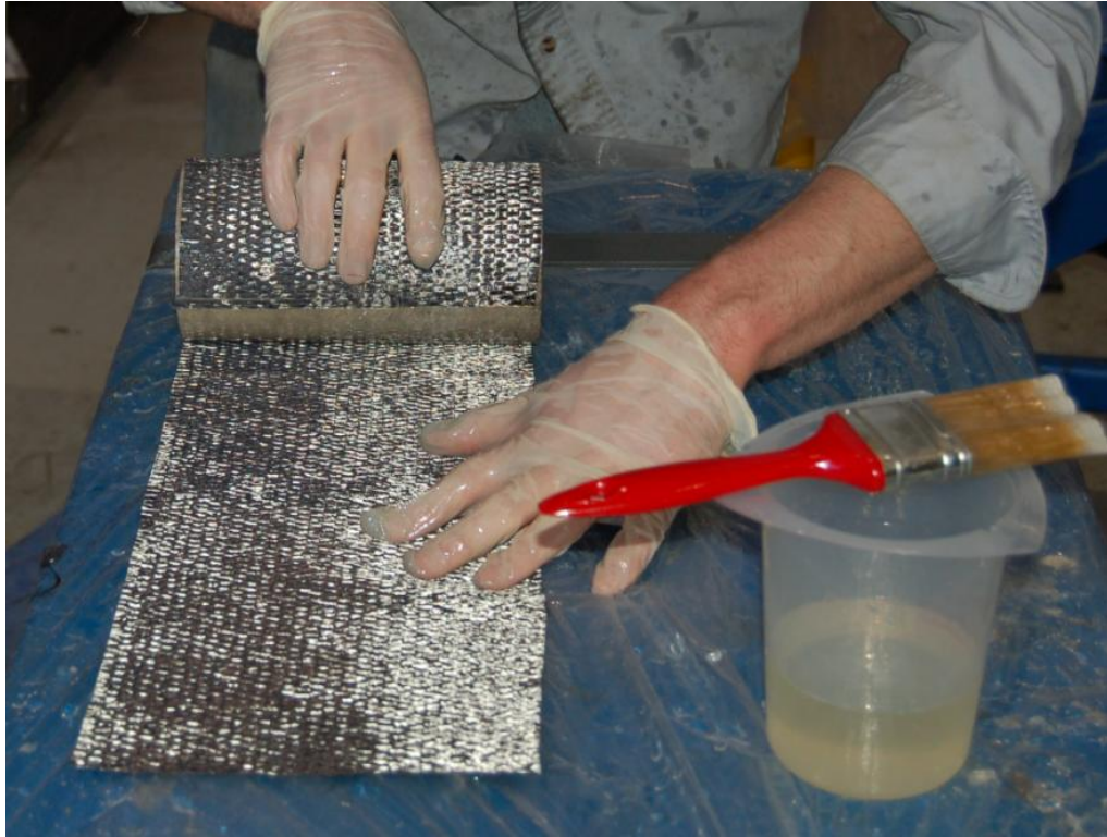
Figure B-3: Application of inner 90° layer to concrete cylinder
