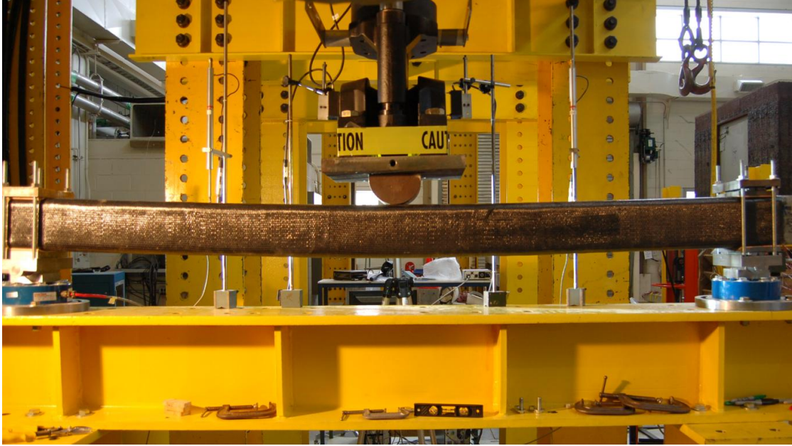
Figure 4-29: QS-2 at peak deflection (29.5 mm) during static testing
