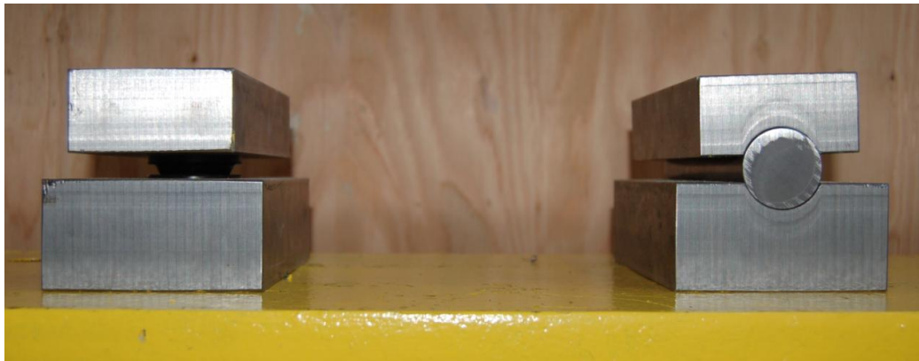
Figure 3-21: Simple supports used in conjunction with prototype axial loading system
