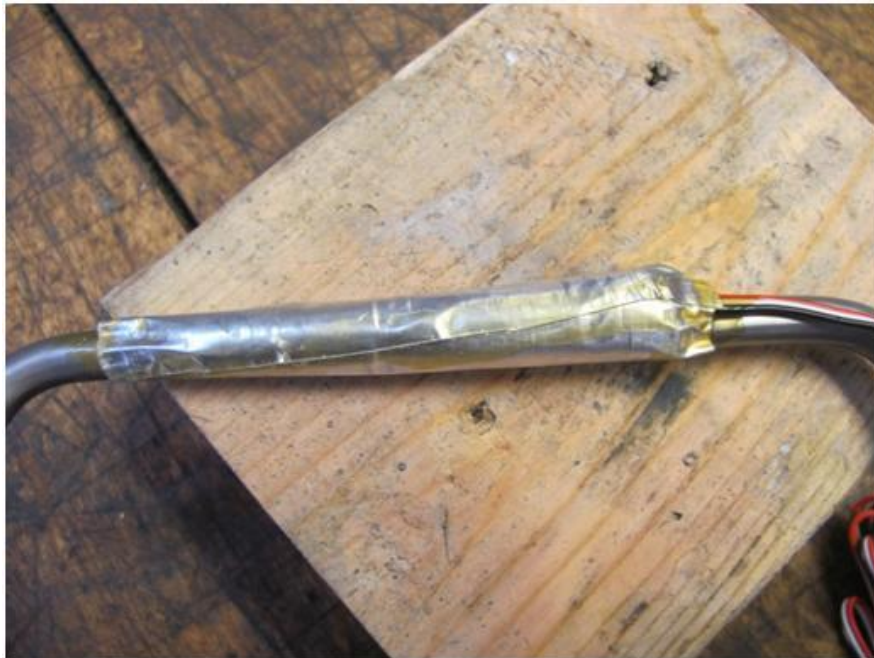
Figure 3-5: Protected and finalized stirrup strain gauge assembly
