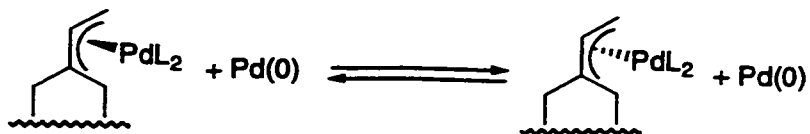
Figure 3-4 cis-trans isomerization by S_N2 displacement of an \pi^3 -palladium complex by a Pd(0) complex.
