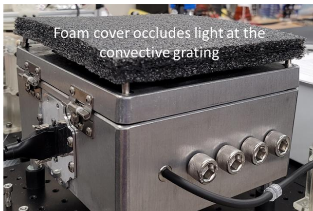
Figure 3.44. SiNx nanopore electrical noise from ambient room light. Ambient light entering the enclosure via the ventilation grating produced significant low frequency noise current spikes on a PSD for a 12 nm nominal thickness SiNx membrane on a Si backbone, assessed at 0 mV in 3.6M LiCl + 10 mM HEPES, pH8 electrolyte. The noise hump in the 10^2 - 10^3 Hz range is related to the use of high capacitance (190 pF) chip with the Chimera amplifier, and not the light source. A simple non-conductive foam cover on standoffs is effective at preventing a significant portion of external ambient light from entering the enclosure via the convective grating in the lid.
