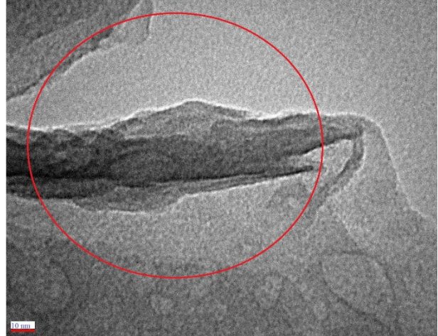
Figure 4.19: A zoomed in view of Figure 4.18 where the EDS analysis is conducted. The thick of the kaolinite nanosheet varies throughout the nanosheet. The red scale bar is 10 nm.
