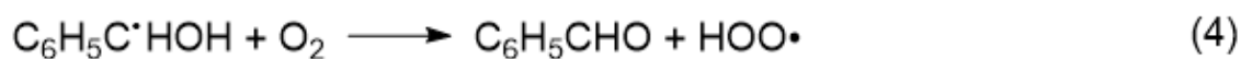
Figure 4.5.1: The oxidation of benzyl alcohol to benzaldehyde: (1) – photoexcitation of decatungstate; (2) - reaction of {}^3\text{DT}^* with benzyl alcohol; (3) - reaction of \text{DTH}\cdot with oxygen; (4) – reaction of benzyl radical with oxygen.
