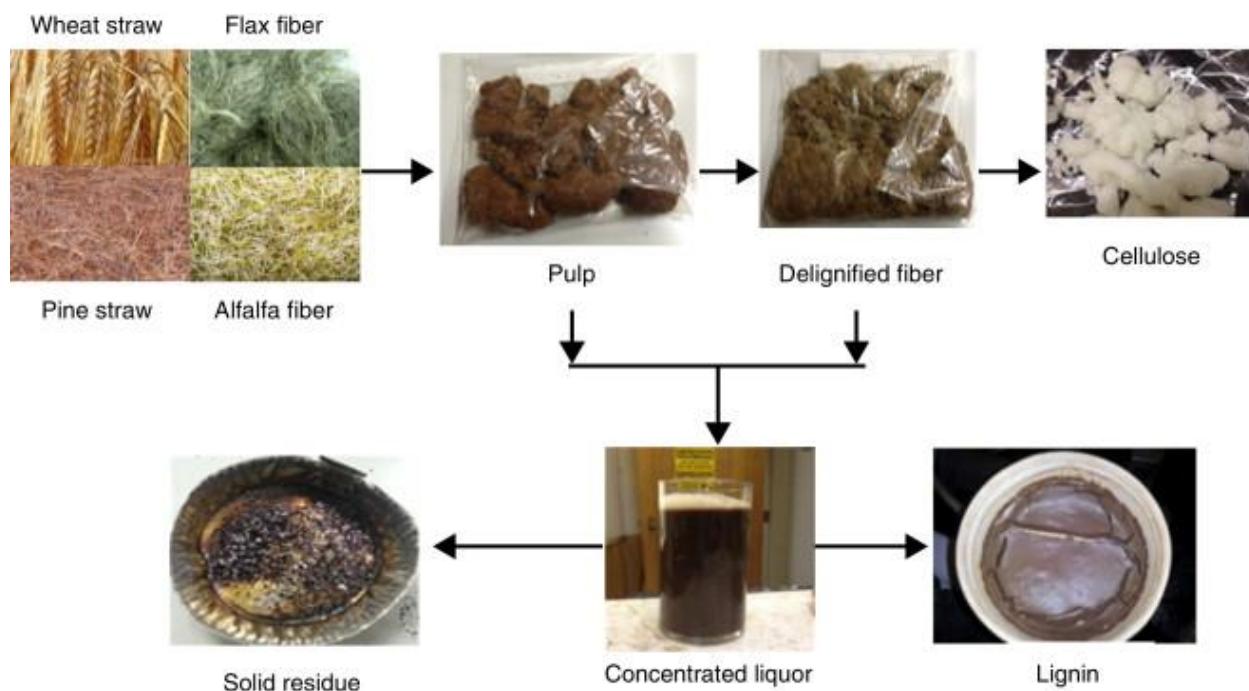
Figure 1.8: Schematic diagram of the organosolv process of lignin extraction. From Watkins et al. 21
