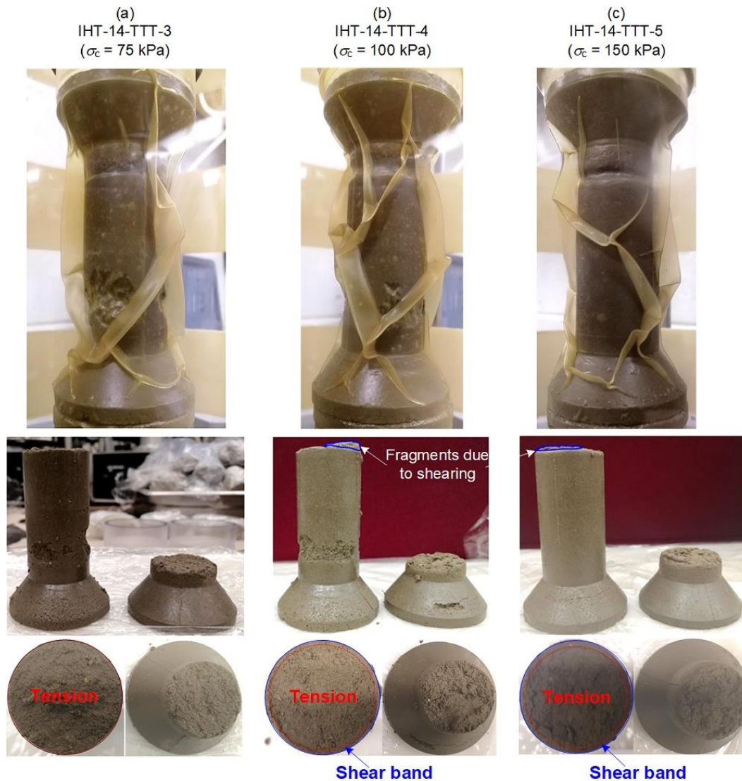
Figure 6.14 Photos of the rupture zone of compacted specimens after the triaxial tensile test: (a) IHT-14-TTT-3, (b) IHT-14-TTT-4, and (c) IHT-14-TTT-5.
