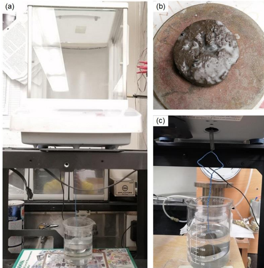
Figure 5.19 (a) Setup for wax immersion method for measuring the specimen volume; (b) Coated soil specimen with wax after dipping into the melted wax; (c) Suspended weight of the wax-coated specimen in kerosene determined by below balance weighing.
