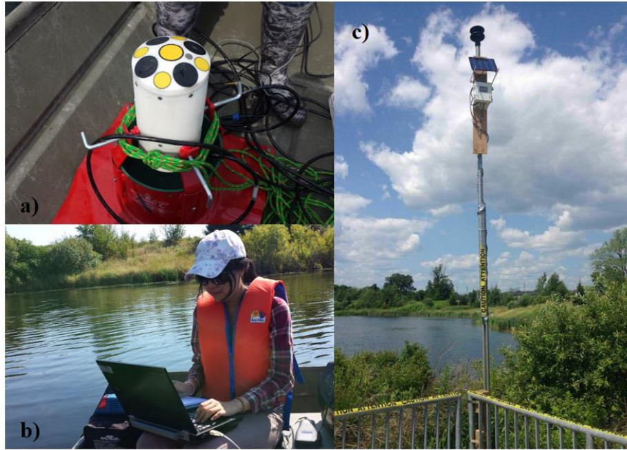
Figure 3.1 a) a stationary mounting system with a secured SonTek RIVERSURVEYOR M9 aDcp unit; b) in the boat collecting data; c) a mounted HOBOWare U30 Station wind logger
