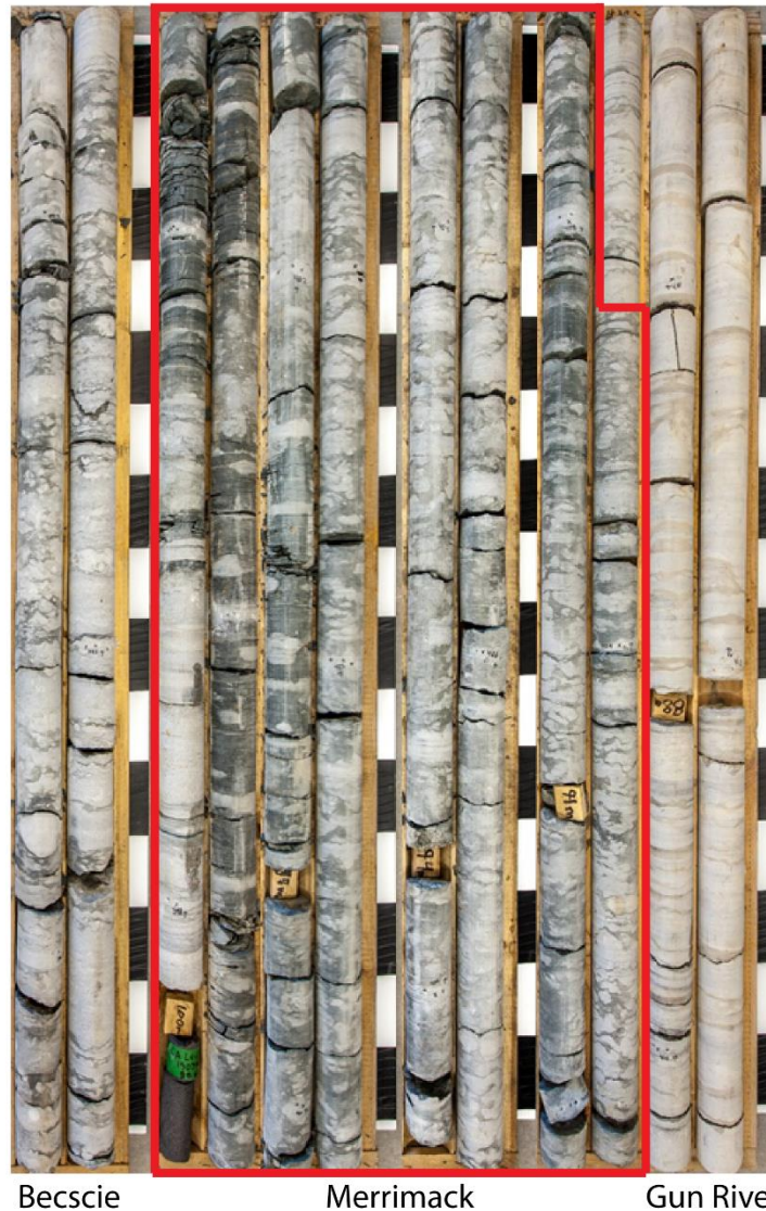
Figure 5.2. Core photograph showing La Loutre #1 boxes # 33 to 28. The Merrimack Formation identified by the red rectangle displays thicker shale interbeds when compared to the underlying Becscie or overlying Gun River formations.
