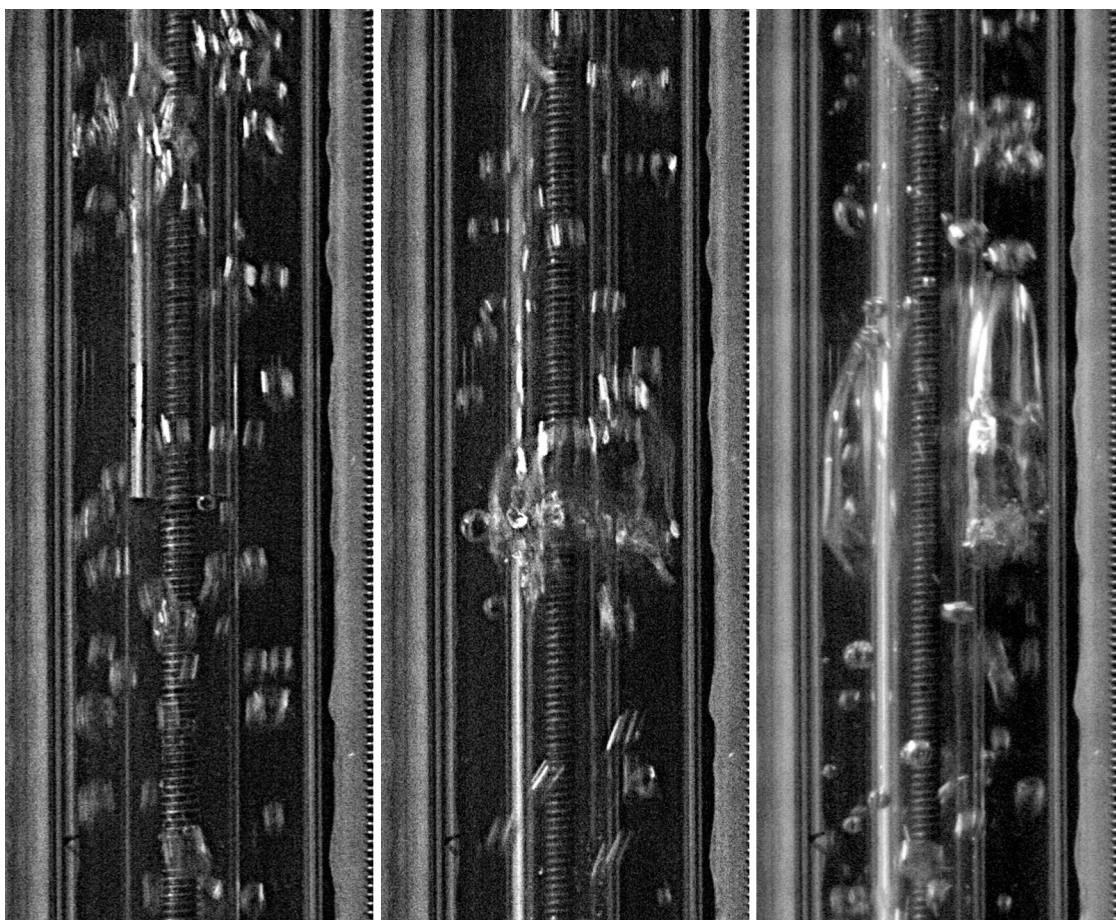
Figure 6.33: Representative images of flow patterns in the bubbly to slug flow transition region for e = 0.3 and j_g = 0.018 m/s: bubbly flow (left, j_l = 0.267 m/s), cap-bubbly flow (centre, j_l = 0.194 m/s) and slug flow (right, j_l = 0.124 m/s).
