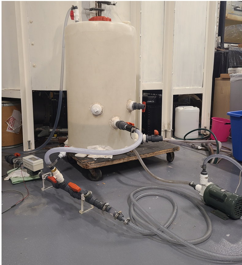
Figure 4.10: A photograph of the separation tank, the pump and the flowmeter used in the flow loop.
