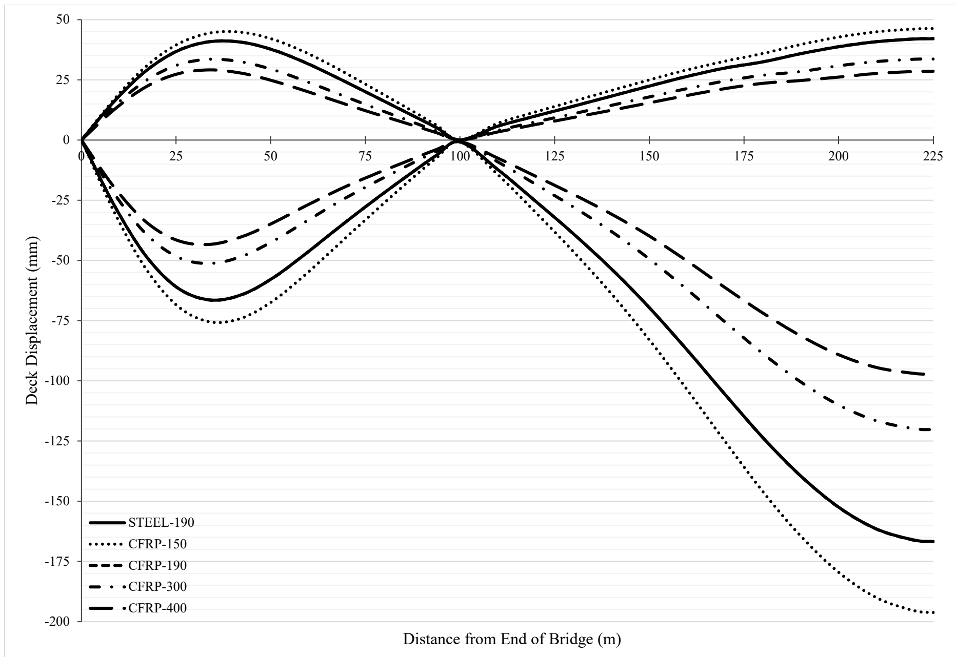
Figure A-8: Minimum and maximum vertical deck displacements under LL ENV
