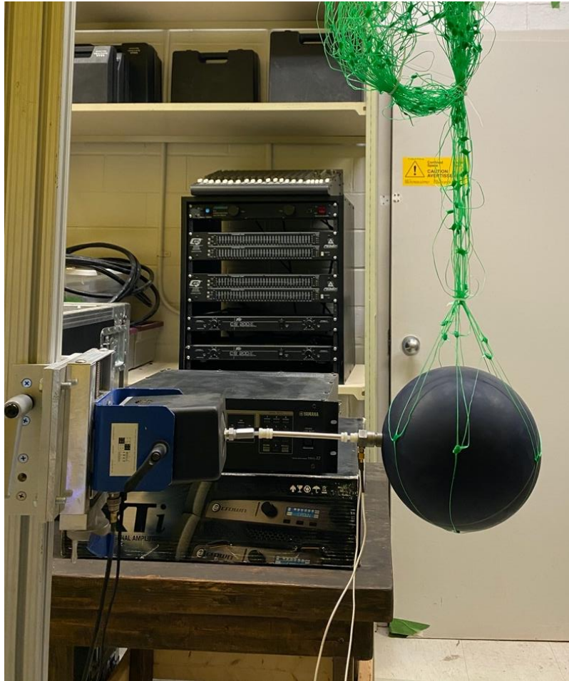
Figure 4.4 Shaker mounted to vertical support during measurement of impact rubber ball.
