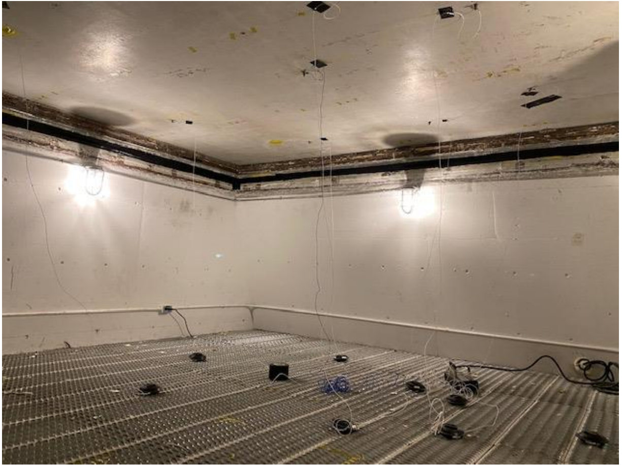
Figure 5.12 Lower chamber during floor testing.
