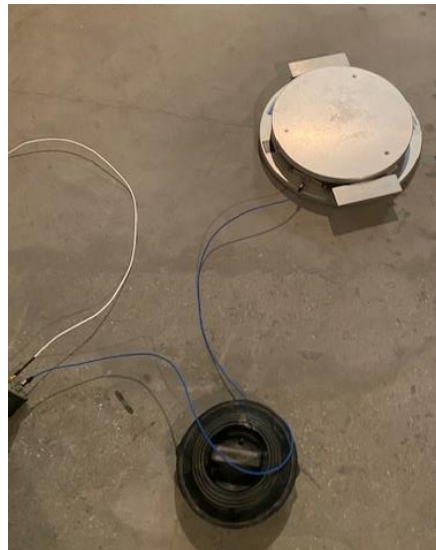
Figure 4.10 The PF-10 force plate resting on a concrete floor
