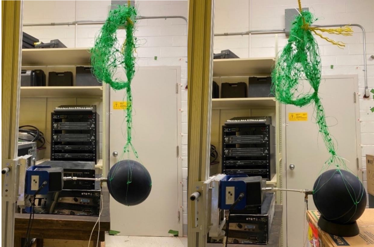
Figure 5.5 Horizontal measurement setups for the mobility of the impact rubber ball, suspended (left) and resting (right).
