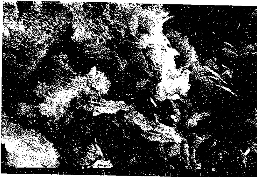
b) Cement+2% \text{Ca}(\text{C}_3\text{H}_5\text{O}_2)_2 \cdot \text{H}_2\text{O} , w/c=0.35, 1 day, paste off glass substrate
