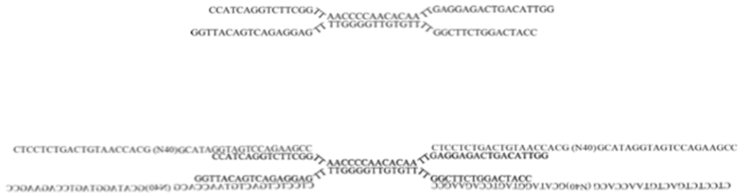
Figure 2.10. Scheme of a quadramer and bridge. The oligonucleotide bridge mediates the formation of the quadramer. Reproduced with permission from 84 .
