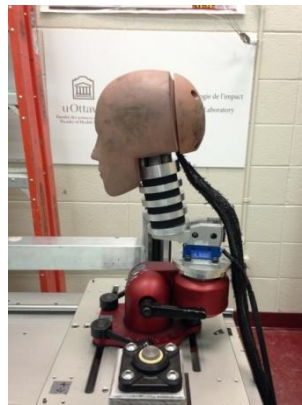
Figure 6. Hybrid III headform attached to unbiased neckform
