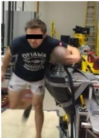
Figure 14. Arm-out shoulder-to-headform tackle using a 3-step approach in the laboratory
