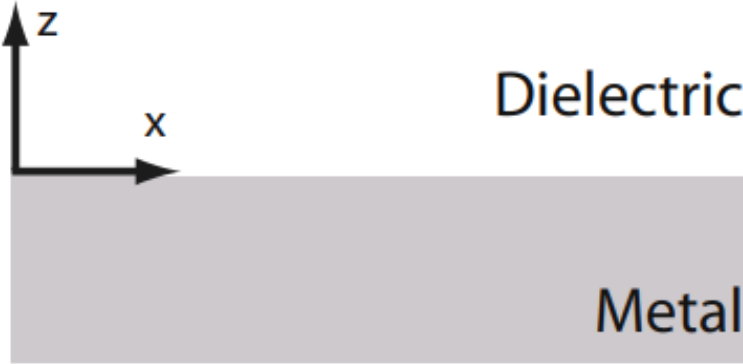
Figure 2.4: Schematic of a metal-dielectric interface, showing the propagation direction of the SPP along the x -axis and the exponential decay in the z -direction [1].
