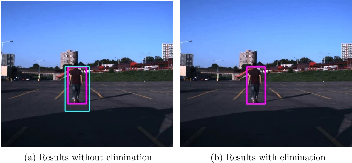
Figure 3.21: Examples of results with and without elimination – the pedestrian in the distance around TSD are detected by both C_s and C_L , the 3.21a is the result without elimination and the 3.21b is the result with elimination.
